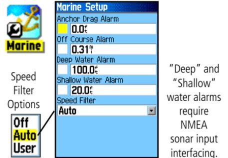
"Deep" and "Shallow" water alarms require NMEA sonar input interfacing.
