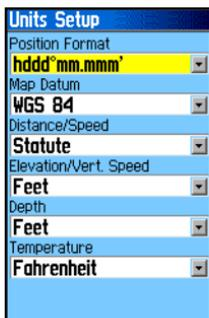
The screenshot shows the 'Units Setup' menu with the following options: Position Format (hddd°mm.mmm'), Map Datum (WGS 84), Distance/Speed (Statute), Elevation/Vert. Speed (Feet), Depth (Feet), Temperature (Fahrenheit), and a status bar showing 10:18:39 AM on 10-NOV-03.
