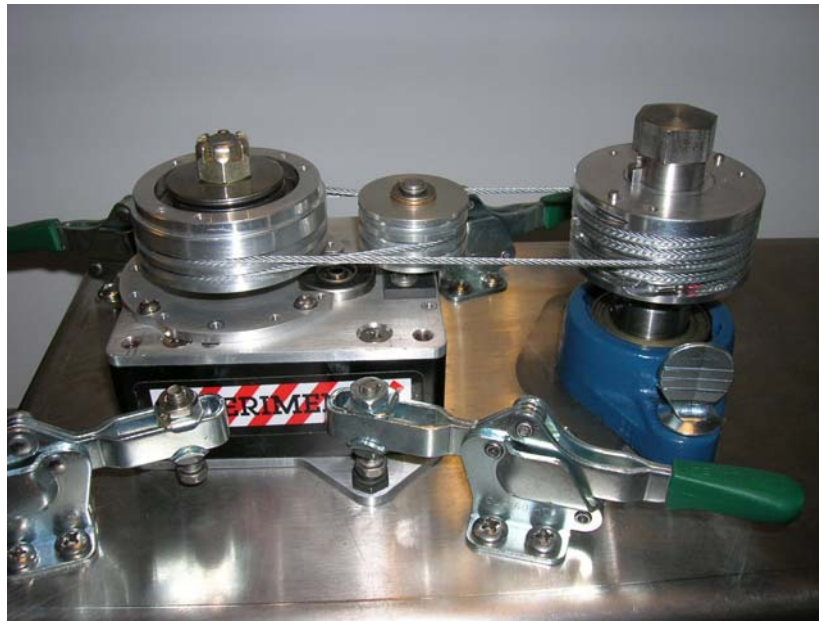
Figure 3-22. Slack taken up, capstan centered
