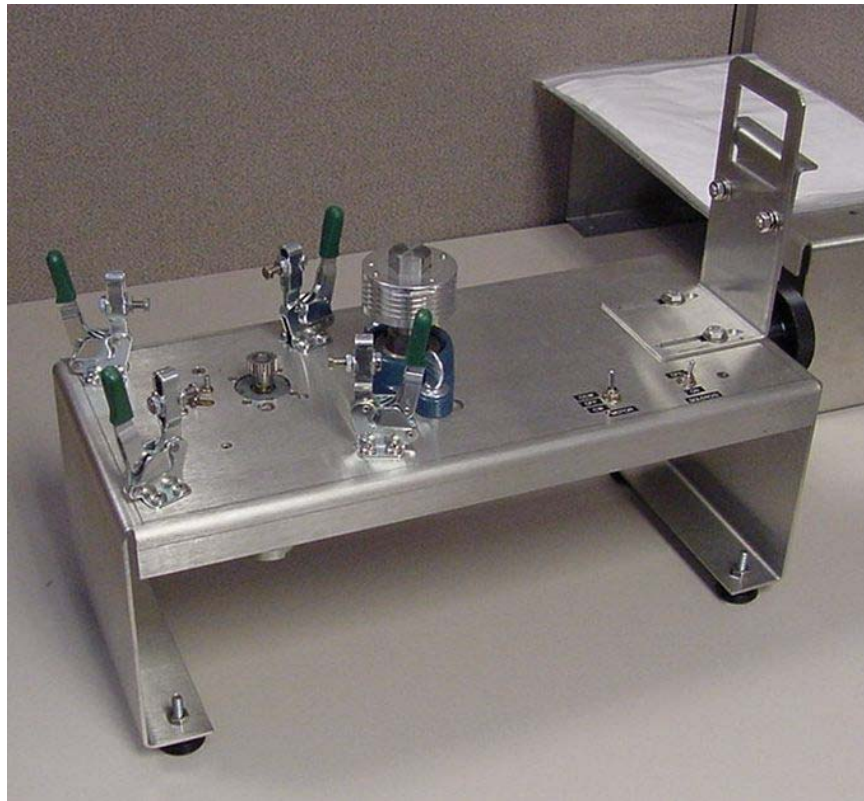
Figure 3-3. Slip-Clutch Adjustment Fixture (P/N T10-00110-01)
