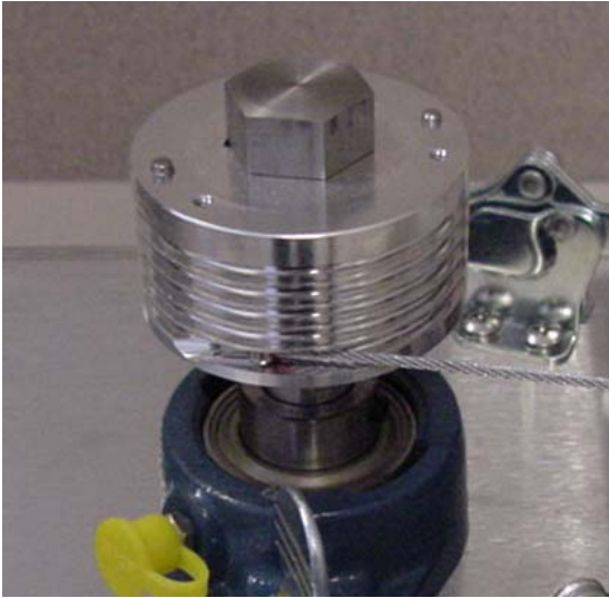
Figure 3-6. Cable Placement (fixture capstan)
