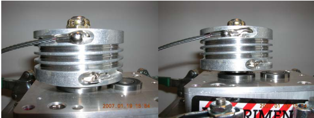
Figure 3-10. Inserting 3/32 cable in the unit capstan.
