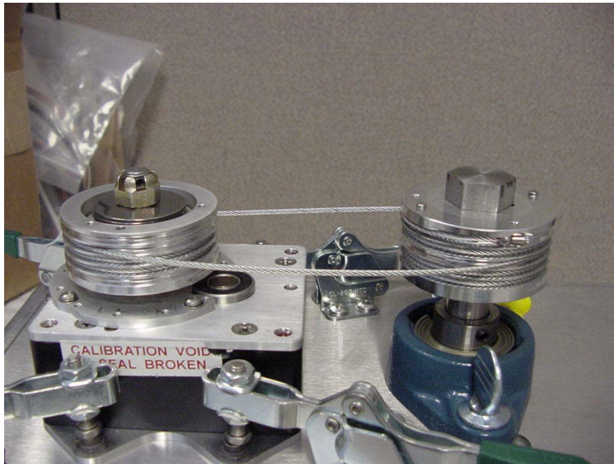
Figure 3-9. Cable End Placement (unit capstan)
