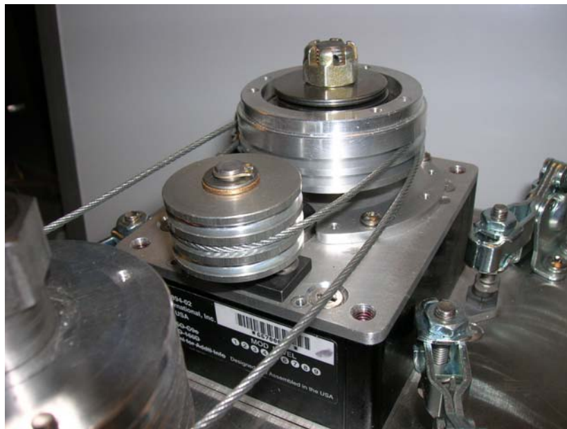
Figure 3-19. Cable wrapped around unit upper slot
