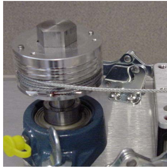
Figure 3-7. Cable Placement (fixture capstan)
