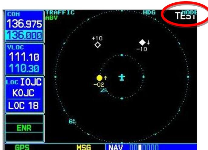
Figure 9. System (Self) Test (GNS 530 Shown)
