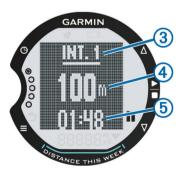
The paused screen includes the interval number ③, interval distance ④, and swim time for the interval ⑤. The screen appears inverted (*Inverting the Display of the Training Pages*, page 4) until you select
