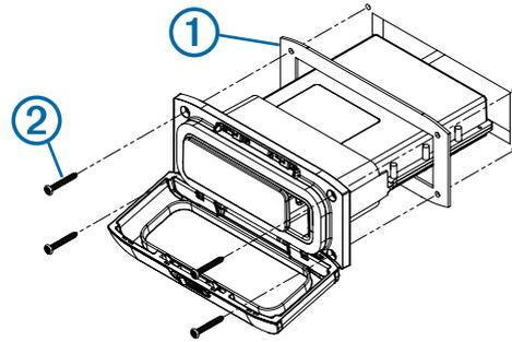
**13** Secure the docking station to the mounting surface using the included screws ②.
