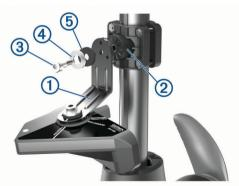
2 Fully tighten the shoulder screw to secure the extension arm to the shaft bracket.
