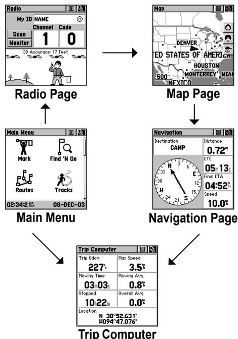
While these five Main Pages provide you with different types of information, they all share common features like Option Menus and a Main Page Menu. Access the Option Menu and Main Page Menu by using the **Thumb Stick** to highlight the on-screen button. Then press the **Thumb Stick In**.
