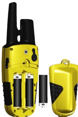
2. Insert batteries observing the polarity reference molded into the unit housing. Orient the negative (-) battery terminal toward the spring.
