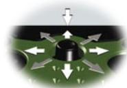
Sometimes you will need to spell out things using the **Thumb Stick** and an on-screen keyboard. To enter characters with the on-screen keyboard, press the **Thumb Stick** Up, Down, Left, or Right to highlight the desired character (letter, number, or a space). Press the **Thumb Stick In** to select that highlighted character. Choose **Back**
