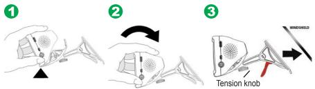
Fit the bottom of your c320 into the cradle of the suction cup mount.
