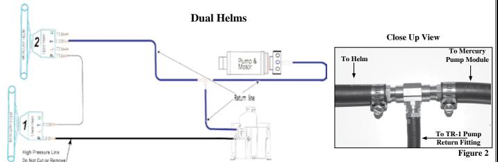
Locate the low pressure return hydraulic hose. It will run from the (T) fitting at the Mercury Helm to the return fitting on the Mercury Pump Module. It is very important that you verify that you have the right hose. You will need to cut this hose and install the barbed tee fitting, as shown in Figure 2.
