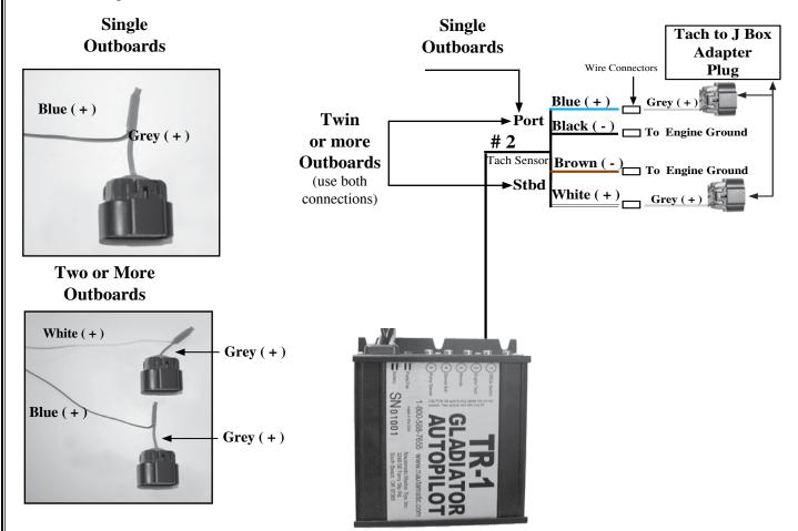
Note: It may be necessary to convert the tach signal from the Mercury Outboard from digital to analog signal. Only a Mercury Service Center may make this change. Please contact technical support at 1-866-559-0229 if you have any questions.
