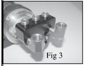
Install the 90 degree fittings into the manifold of the pump as shown in Fig 3. Use a Loctite "Pro Lock" tight multi-purpose anaerobic gel, part number 51604, or equivalent on **pipe threads only** (see fig 8) Tighten fittings securely.
