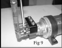
Mount the Valve Assembly 90 degree fittings directly into the manifold, using care not to cross thread them in the holes (use appropriate anaerobic gel on threads). Align tees and tighten fittings securely. See Fig 9.
