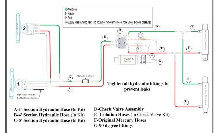
**Note:** Depending on the type of installation used for the Check Valve the 90 degree fittings (G) may be optional in the pump Manifold.
