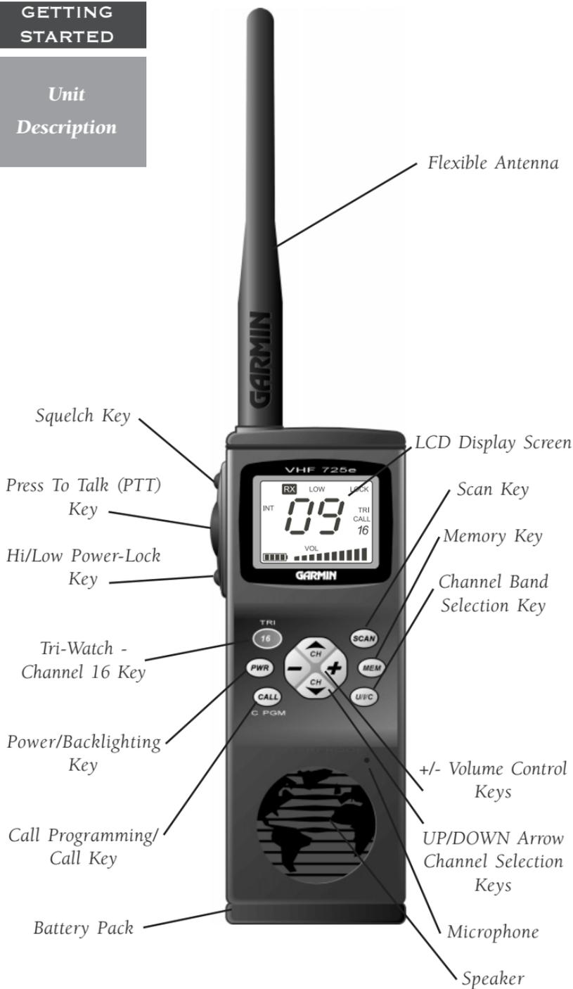
The VHF 725e is a 5 watt marine VHF communications transceiver in a convenient handheld package.
