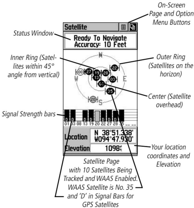
The Satellite Page provides a picture of satellite signal tracking, tells you when the unit is ready for navigation, and shows your location coordinates.
