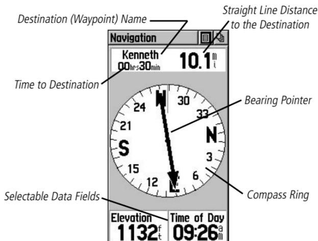
The Navigation Page provides active guidance with a rotating compass ring that shows your course over ground (track) while you're moving and a bearing pointer to indicate the current direction to your destination (bearing) relative to the course over ground.
