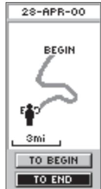
The 'BEGIN' point is the point defining the starting point when saving a track log. 'END' is the last point that was saved. Each saved track will always have a 'BEGIN' and 'END' point for navigation. The 'BEGIN-END' pair imply the direction of the saved track. If you want to retrace the track, navigate to 'END'. If you want to track back to the starting point, navigate to 'BEGIN'.
