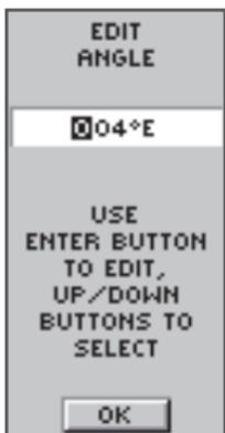
To manually set the variation or declination, highlight the Angle field, press **ENTER** and input a new angle.
