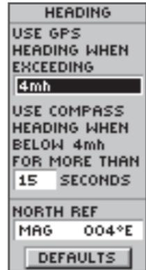
The eTrex Summit can be set to disable the Electronic Compass above a user selected speed. This helps to conserve battery power.
