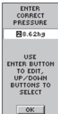
The eTrex Summit can automatically calibrate the altimeter using GPS altitude. For optimum performance of the Altimeter, you should perform the calibration procedure entering either the correct elevation or barometric pressure.
