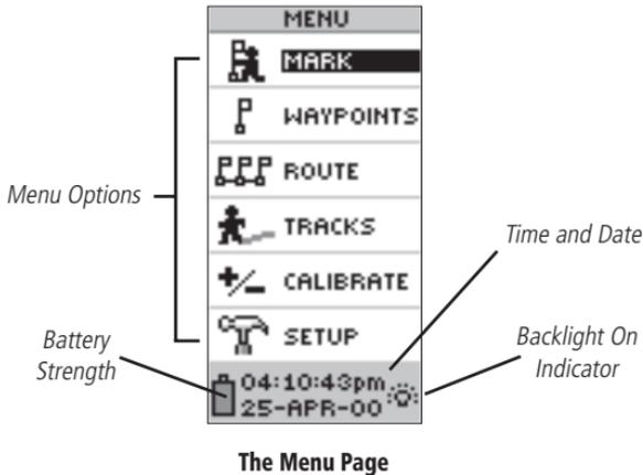
The Menu Page gives you access to eTrex Summit's more advanced features. With the Menu Page you can create and view waypoints, create a route and view track logs, calibrate the electronic compass and altimeter or access the system setup features. Information on each of these advanced features is included in the Reference Section of this manual.
