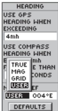
The eTrex Summit automatically adjusts the variation/declination. While it should rarely be needed the user can manually adjust the variation/declination.
