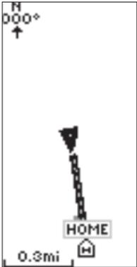
When you select 'Orient Map Northwards' the figure icon is replaced by a 'direction' triangle.
