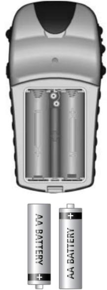
*Remove the batteries from your eTrex Summit if you don't expect to use it for several months. Be sure to observe the proper polarity when inserting the batteries. Follow the battery manufacturer's instructions on the proper care and handling of the batteries.*
