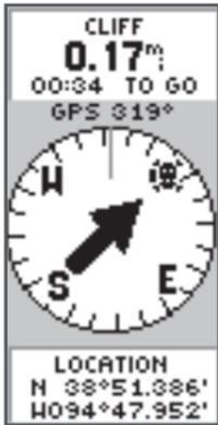
The pointer tells you what direction you should move. When the pointer is pointing right, just move right until the pointer is pointing straight up and points to the moving direction line (see picture below).
