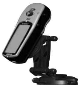
While mounted in a car or on a cycle the eTrex Summit will be tilted enough for the Electronic Compass to become inaccurate. The eTrex Summit will automatically switch to a GPS heading when you exceed 10 mph. To switch back to the compass press and hold the **PAGE** key or wait 90 seconds after slowing below 10
