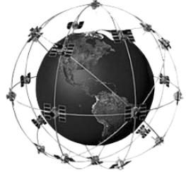
The orbital paths of these satellites take them between roughly 60 degrees North and 60 degrees South latitudes. What this means is you can receive satellite signals anywhere in the world, at any time.
