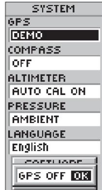
When the unit is in 'DEMO' mode, a warning will appear indicating that the GPS receiver is turned off.
