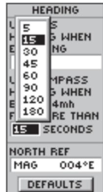
Set a time delay before switching to the electronic compass when moving at a speed slower than the user-selectable speed.
