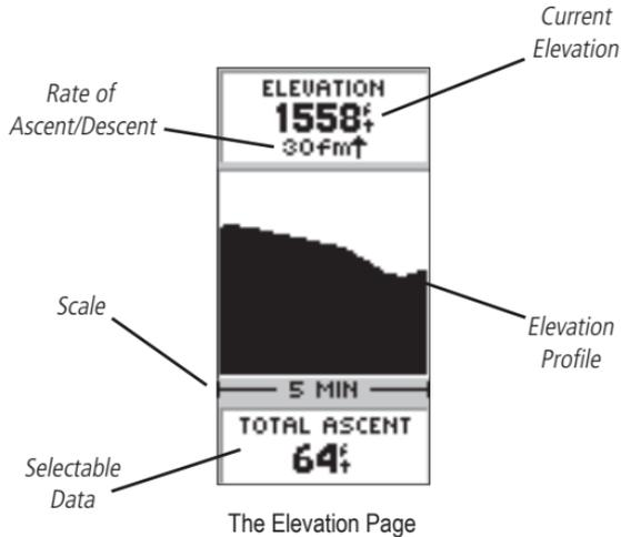
The Elevation Page will provide the user with the current elevation, rate of ascent/descent, and a profile of elevation changes over distance or time. The **UP** or **DOWN** Buttons can be used to scroll through a variety of user selectable data including Pressure, Vertical Speed, Max Descent, Max Ascent, Avg Descent, Avg Ascent, Total Descent, Total Ascent, Min Elevation, Max Elevation, and 12 Hour Pressure Trend.
