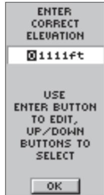
The 'ENTER CORRECT ELEVATION' Page allows you to change the elevation for the waypoint.
