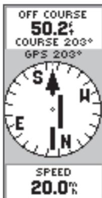
When using the 'Set Course' feature, the 'Pointer' indicates a direct bearing to your destination. The center of the pointer (D-Bar) will show your cross track (the distance you are right or left of the desired course). The example above shows that you are headed toward your destination but have drifted off course to the left about 50 feet. To return to your desired course turn toward the D-Bar (right) until the D-Bar aligns with the pointer
