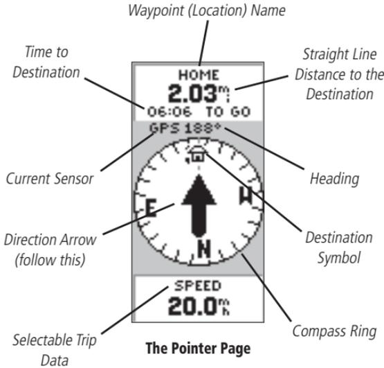
The Pointer Page helps guide you to a destination. When you're moving towards a specific destination, the Pointer Page shows you the name of the location, the distance, time to go and displays a direction arrow in the Compass Ring. To navigate, simply follow the arrow. If the arrow is pointing right, turn right until the arrow is pointing directly ahead and you will arrive at your destination.
