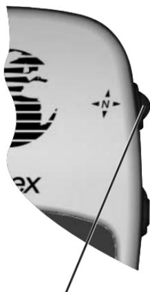
Press and hold the **PAGE** key to activate the compass and display the Pointer Page
