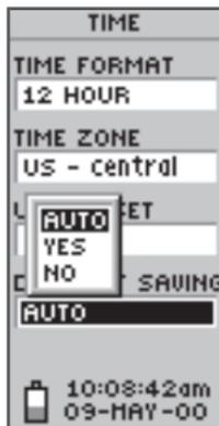
The eTrex Summit can automatically select the Daylight Savings Time mode.
