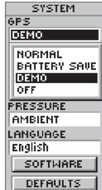
Turn the GPS receiver off to conserve power when using as a compass or developing a pressure trend.
