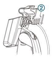
There is an audible click when the locking bracket is installed correctly.
