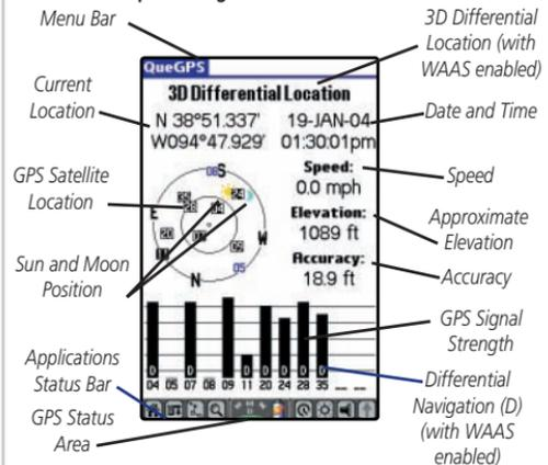
Four or more satellite signals of sufficient strength are required to generate a 3D location fix
