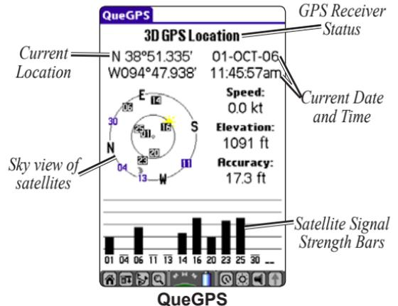
A sky view array in the center, left of the iQue 3600a screen represents the position of satellites in the sky overhead. Your position is represented by the center of the two circles. The outer circle represents the horizon while the inner circle a position  $45^\circ$  from the horizon. The numbers displayed indicate the number assigned to those satellites.
