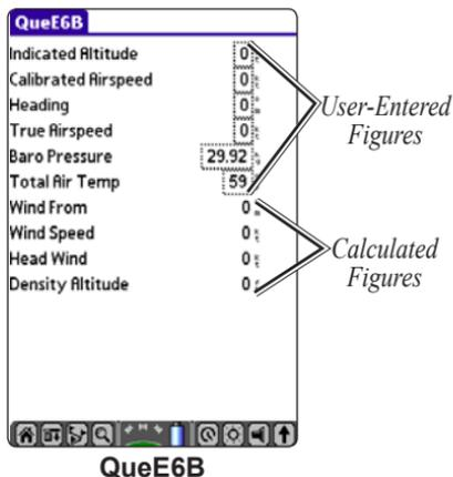
**Indicated Altitude**—required entry for density altitude/true airspeed calculation. Enter the aircraft’s altimeter reading.
