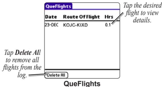
3. Tap the desired flight to view Flight Details. When in the Aviation Cradle, use the **Rocker** key to highlight the desired flight and press **ENTER** to view Flight Details.
