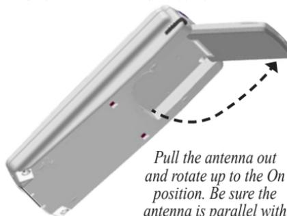
*Pull the antenna out and rotate up to the On position. Be sure the antenna is parallel with the horizon.*
