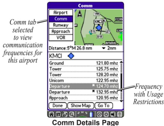
3. Use the **Rocker** key to highlight any frequency with usage restrictions (as denoted by an asterisk) and press **ENTER**. A Usage Restrictions page appears describing the restrictions for the selected frequency.
