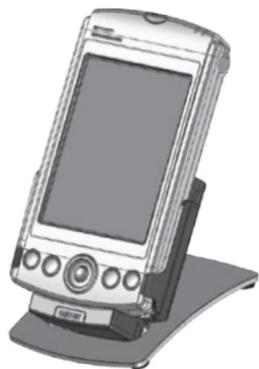
**Note:** You may see a “Backup Battery Very Low” warning, even after you have charged the lithium-ion battery completely. This warning relates to the internal memory battery, which retains data when the main battery is removed. It may take up to two days to charge the internal memory battery completely. During this time, you can still use your iQue M5 out of the cradle.
