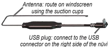
3. Route the antenna on the windscreen and secure it using the suction cups. For best results, route the antenna vertically.
