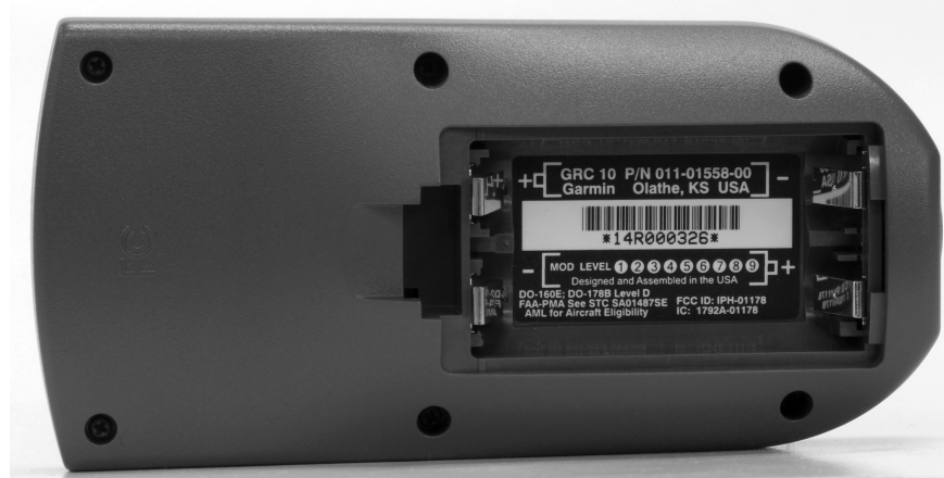
Figure 6-3 GRC 10 Remote Control Battery Department
