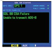
ADS-B STATUS page, lists some of the problems with the ADS-B, that might cause the failure.
