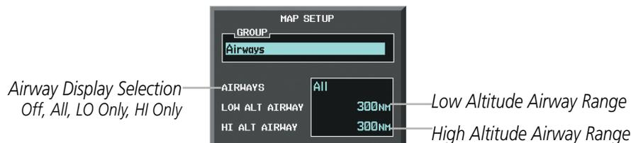
**Figure 5-23 Navigation Map Setup Menu - AIRWAYS Setup**
