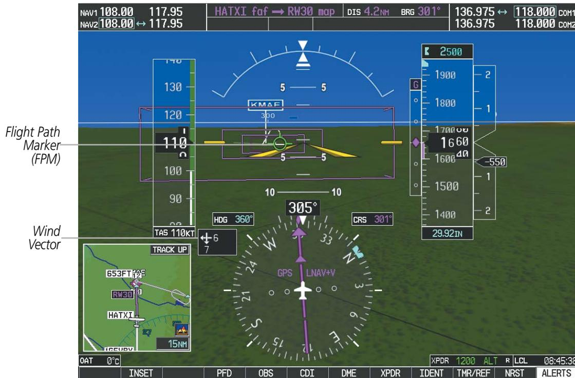
Figure 8-7 Flight Path Marker and Pathways
