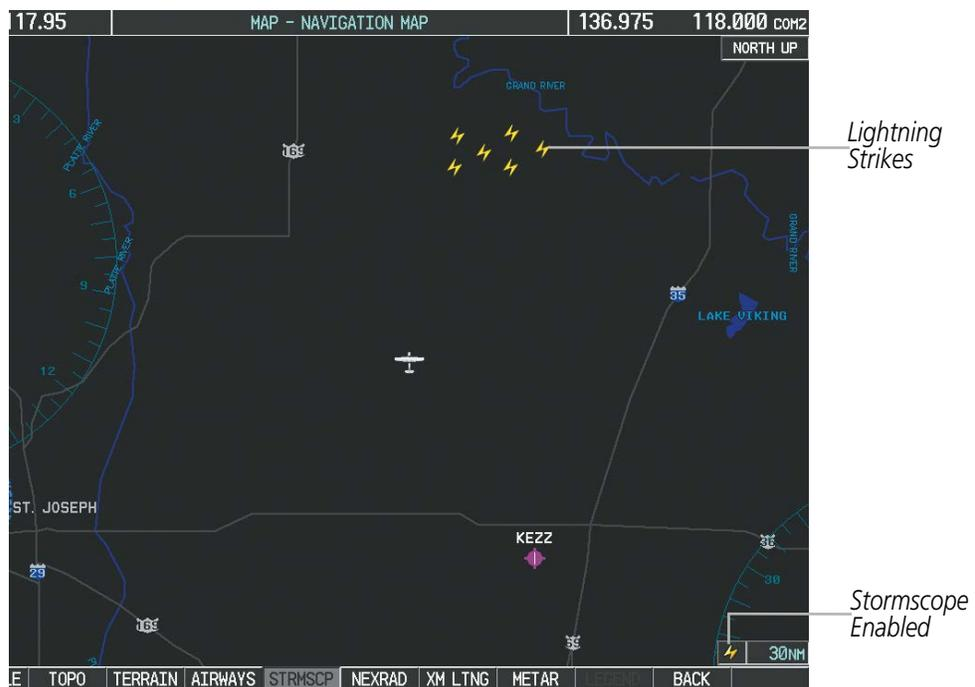
Figure 6-113 Navigation Map Page with Stormscope Lightning Data
