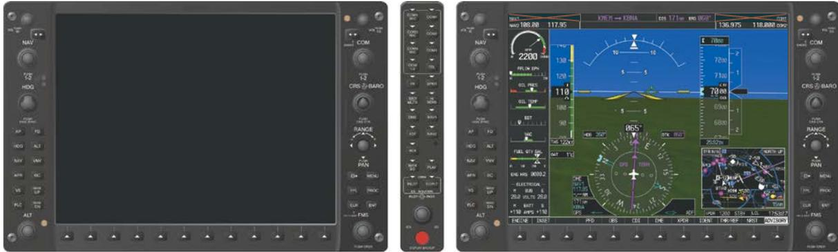
**Figure 1-10 Reversionary Mode (Failed PFD)**
