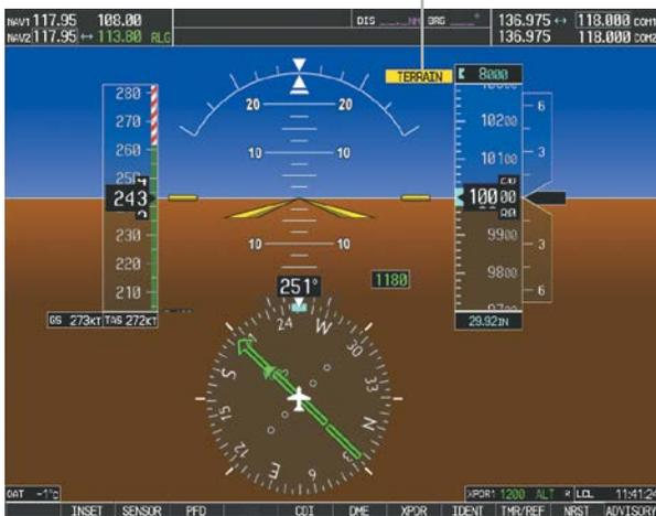
Figure 6-144 TAWS-B PFD Alert Annunciation
