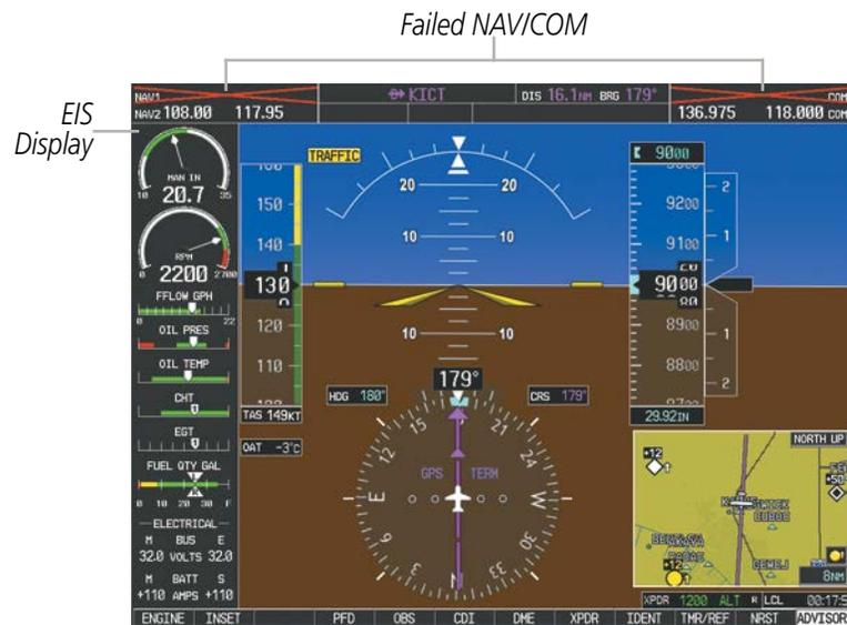
Figure 3-2 Primary Flight Display (182T Reversionary Mode)
