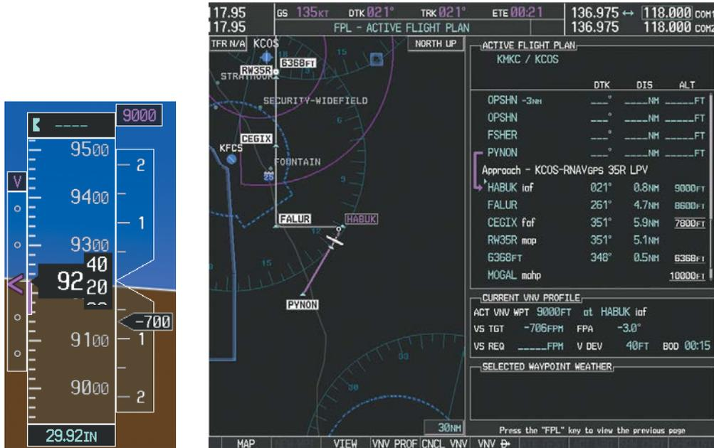
Figure 5-145 Descending Turn to the Initial Approach Fix (IAF)
