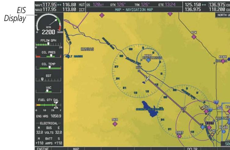
Figure 3-1 Multi Function Display (172S Normal Operations)
