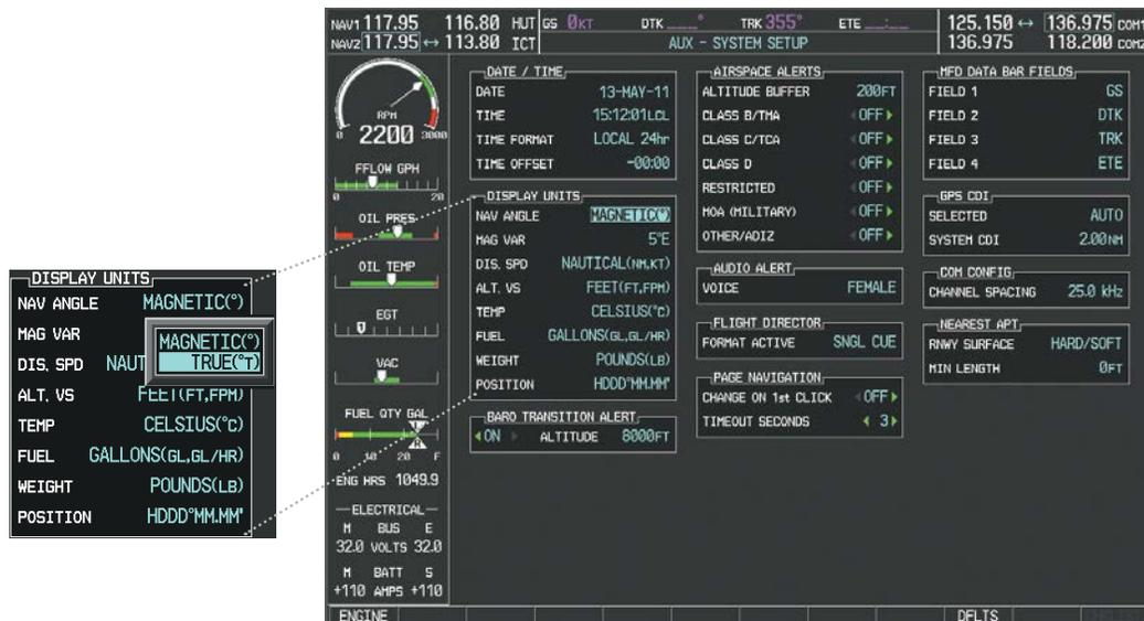
Figure 2-16 Navigation Angle Settings (AUX - System Setup Page)
