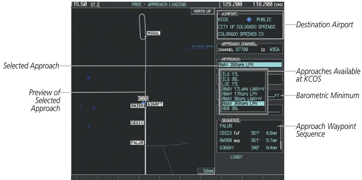
Figure 5-74 Approach Loading Page - Selecting the Approach
