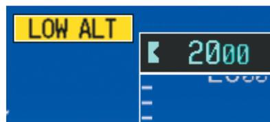
Figure 2-37 Low Altitude on GPS SBAS Approach
