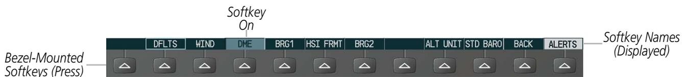
**Figure 1-14 Softkeys (Second-Level PFD Configuration)**
