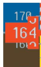
Figure 2-4 Red Pointer Showing Overspeed (Model 172R)
