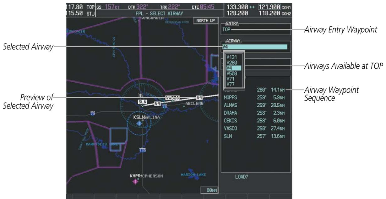
Figure 5-64 Select Airway Page - Selecting Airway
