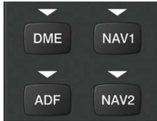
Figure 4-18 Selecting a NAV Radio Receiver
