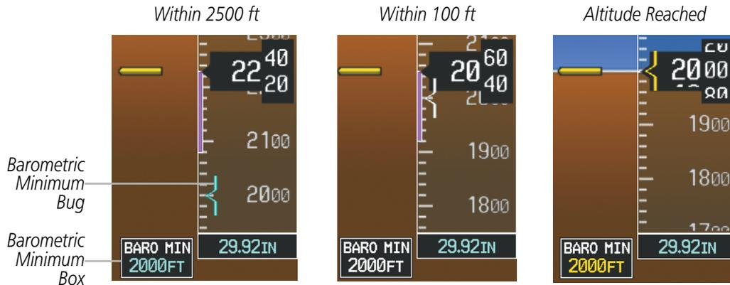
Figure 2-38 Barometric MDA/DH Alerting Visual Annunciations
