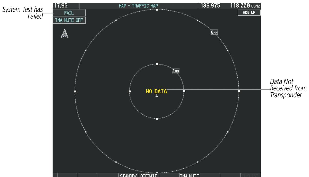
**Figure 6-160 TIS Power-up Test Failure**
