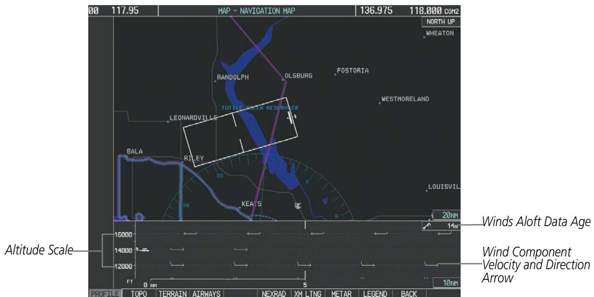
Figure 6-84 Navigation Map Page with Winds Aloft Data on Profile View
