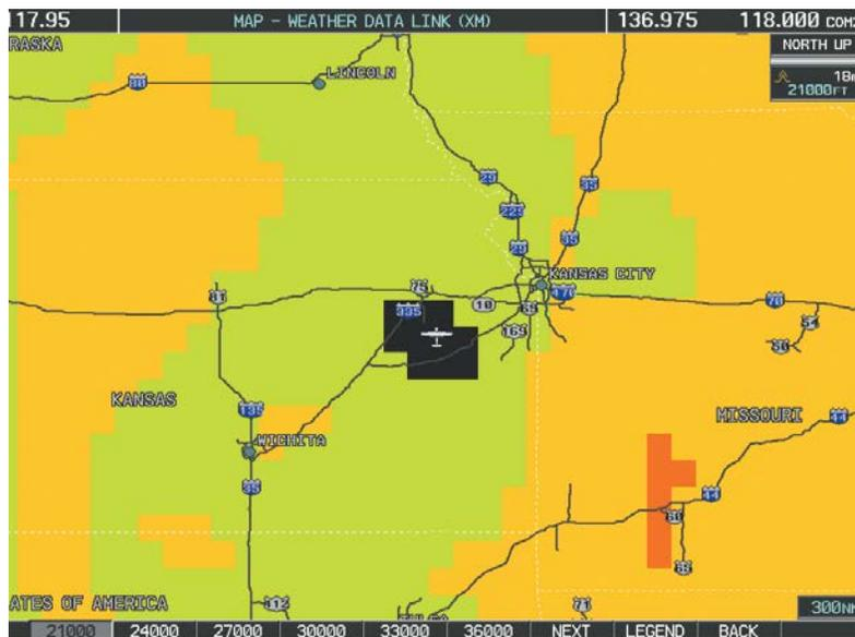
Figure 6-44 Turbulence Data at 21,000 Feet
