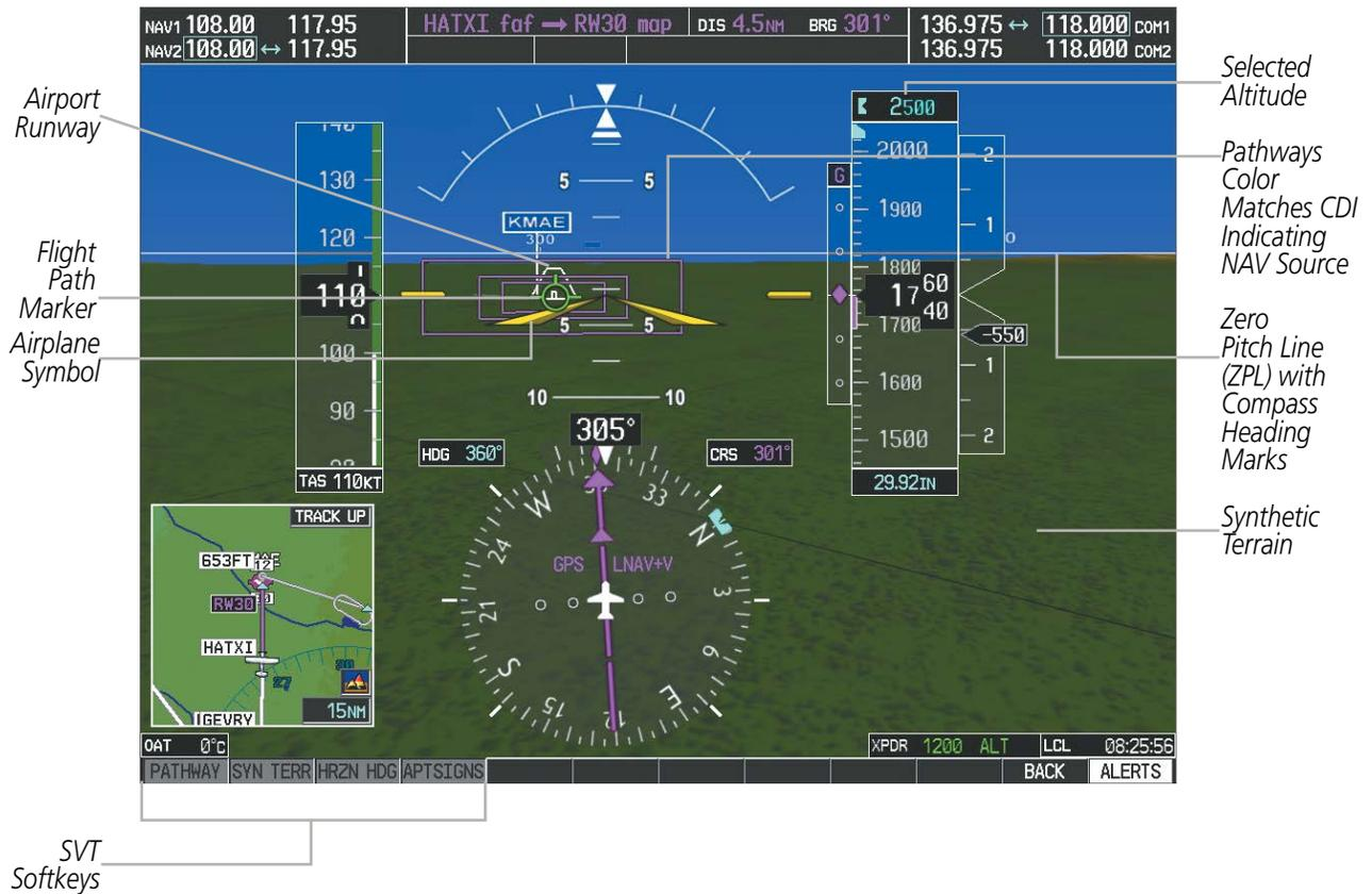
Figure 8-3 SVT on the Primary Flight Display
