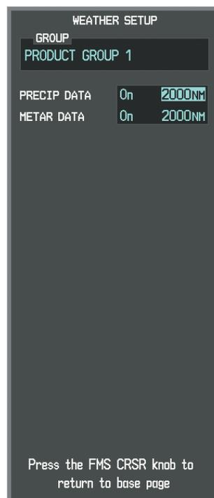
Figure 6-102 Weather Data Link (FIS-B) Page Setup Menu
