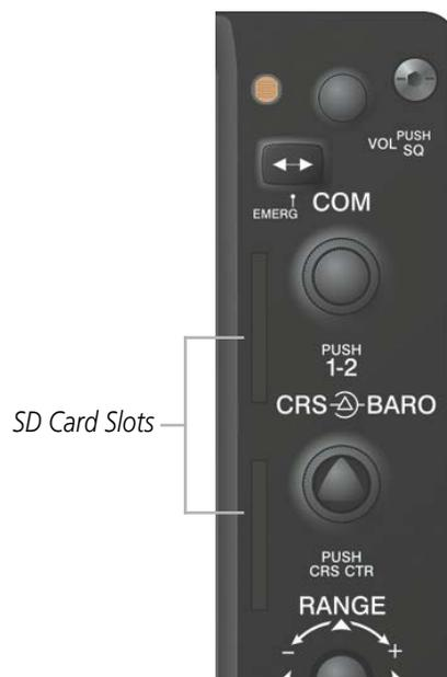
Figure 1-6 Display Bezel SD Card Slots
