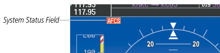
Figure A-4 AFCS System Status Field
