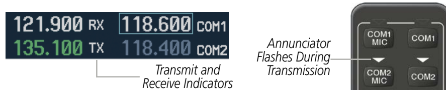
Figure 4-4 COM Radio Transmit and Receive Indications
