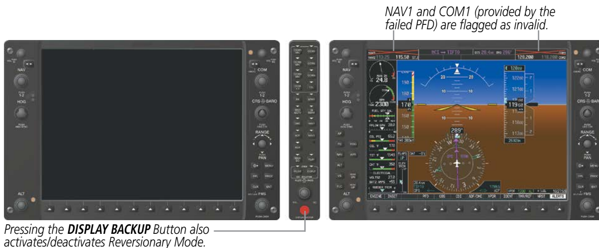
Figure 1-7 G1000 Reversionary Mode (Failed PFD)
