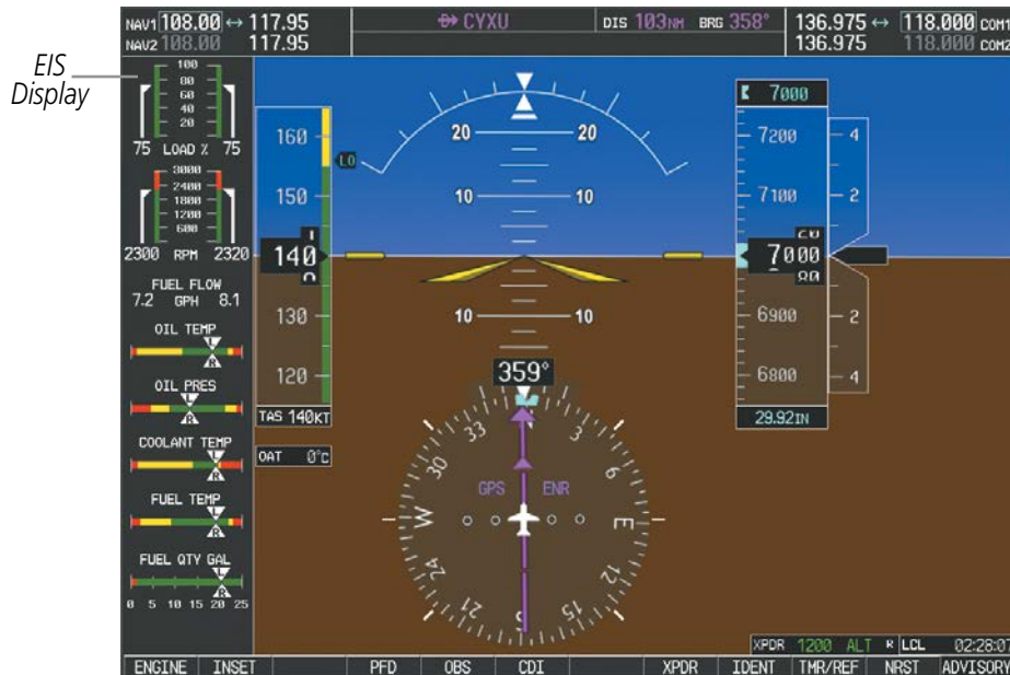
Figure 3-2 Primary Flight Display (Reversionary Mode)
