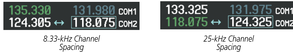
Figure 4-13 COM Channel Spacing
