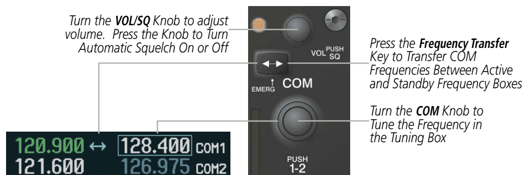
Figure 4-5 COM Frequency Tuning
