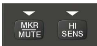
Figure 4-28 Marker Beacon Keys
