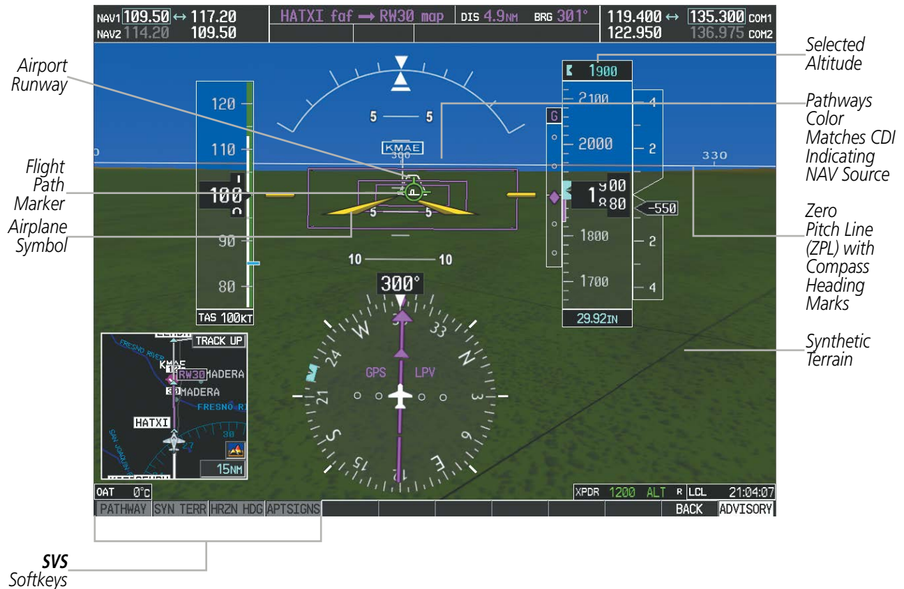
Figure 8-3 SVS on the Primary Flight Display
