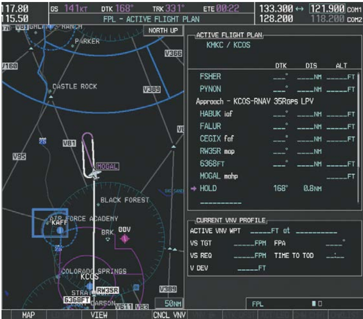
Figure 5-140 Establishing the Holding Pattern
