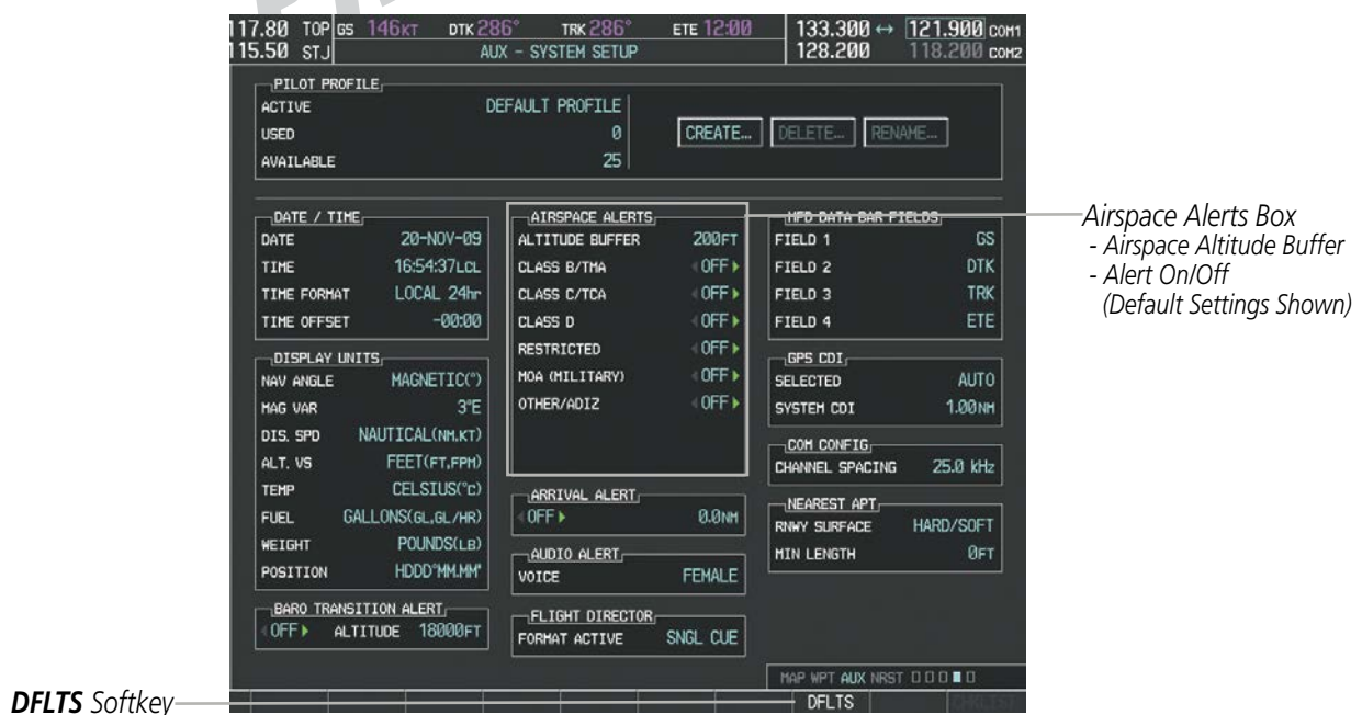
Figure 5-47 System Setup Page - Airspace Alerts
