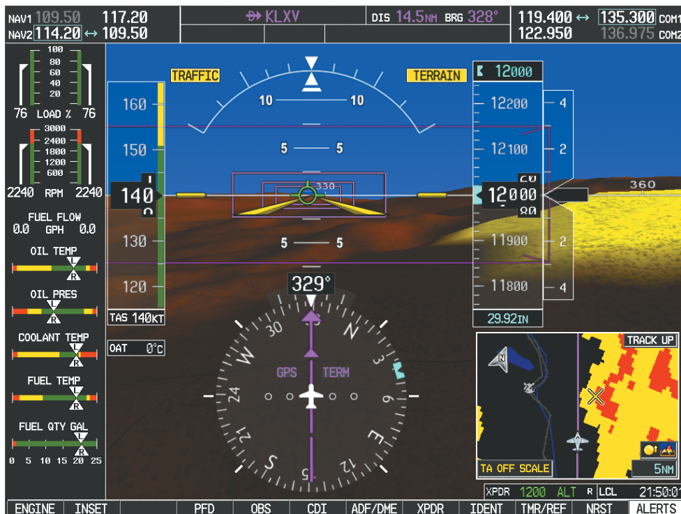
Figure 8-80 SVS Reversionary Mode
