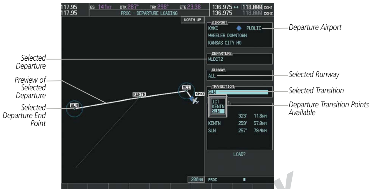
Figure 5-65 Departure Loading Page - Selecting Transition
