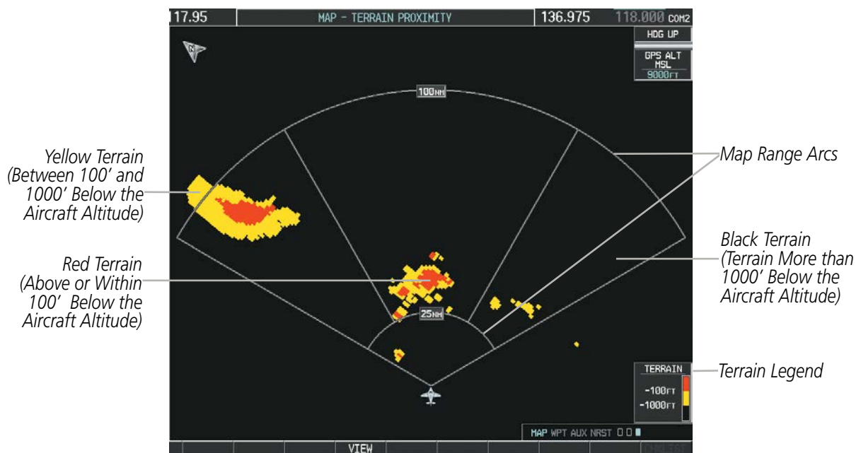
Figure 6-70 Terrain Proximity Page (Arc View)
