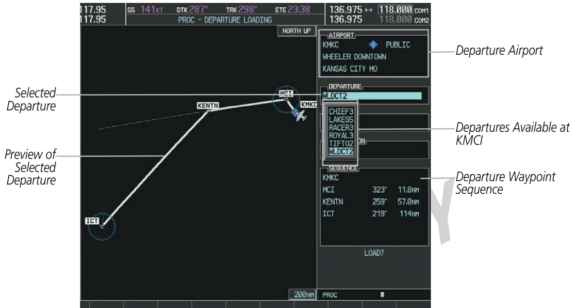
Figure 5-64 Departure Loading Page - Selecting the Departure
