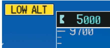
Figure 2-35 Low Altitude on GPS SBAS Approach
