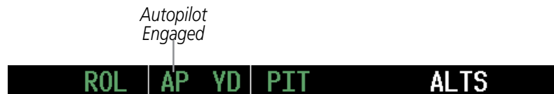
Figure 7-26 Autopilot and Yaw Damper Engaged
