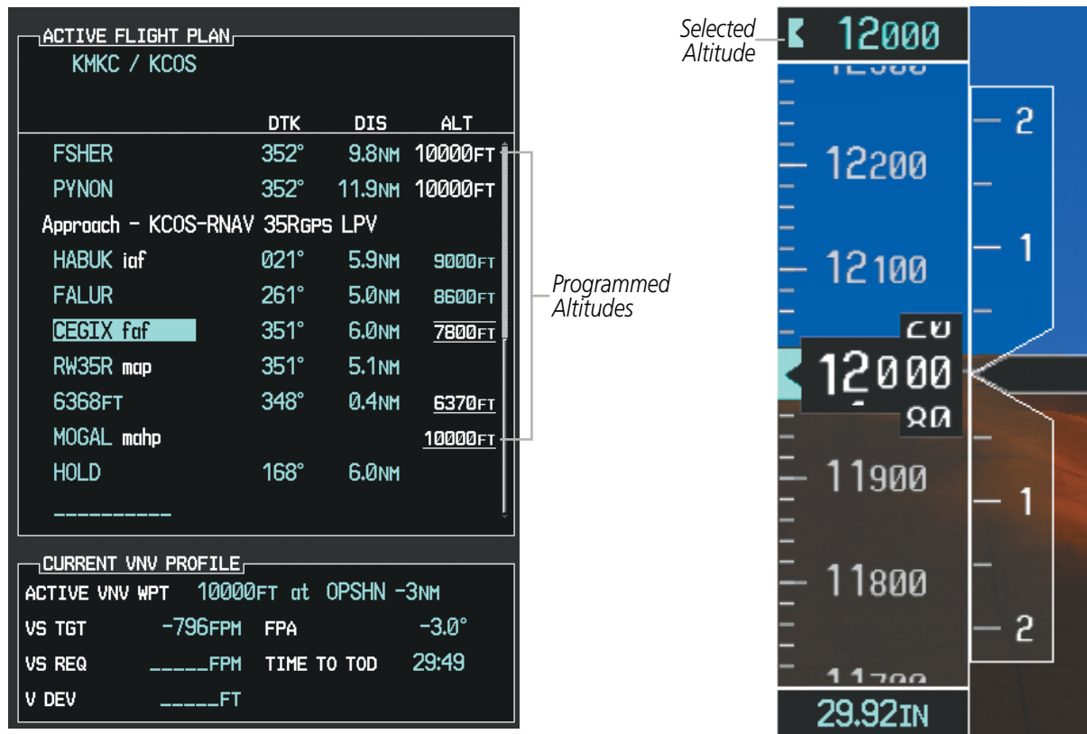
Figure 8-4 Programmed and Selected Altitude
