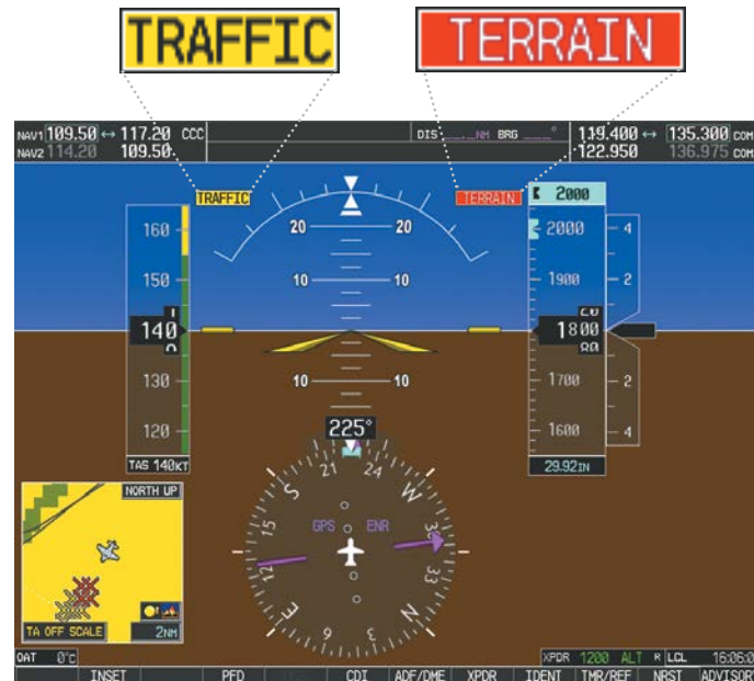
Figure 2-33 Traffic and TERRAIN-SVS Annunciations
