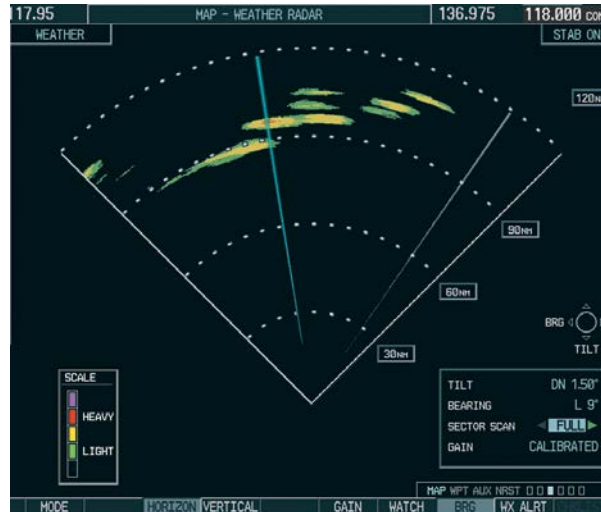
Figure 6-59 Selecting Sector Scan Position
