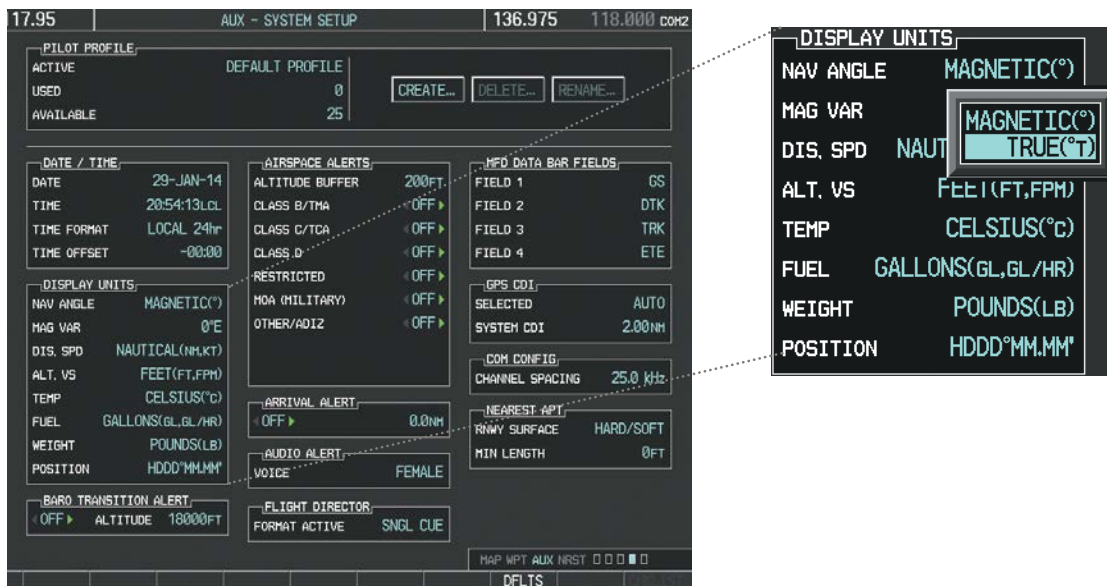
Figure 2-14 System Setup Page, Navigation Angle Settings
