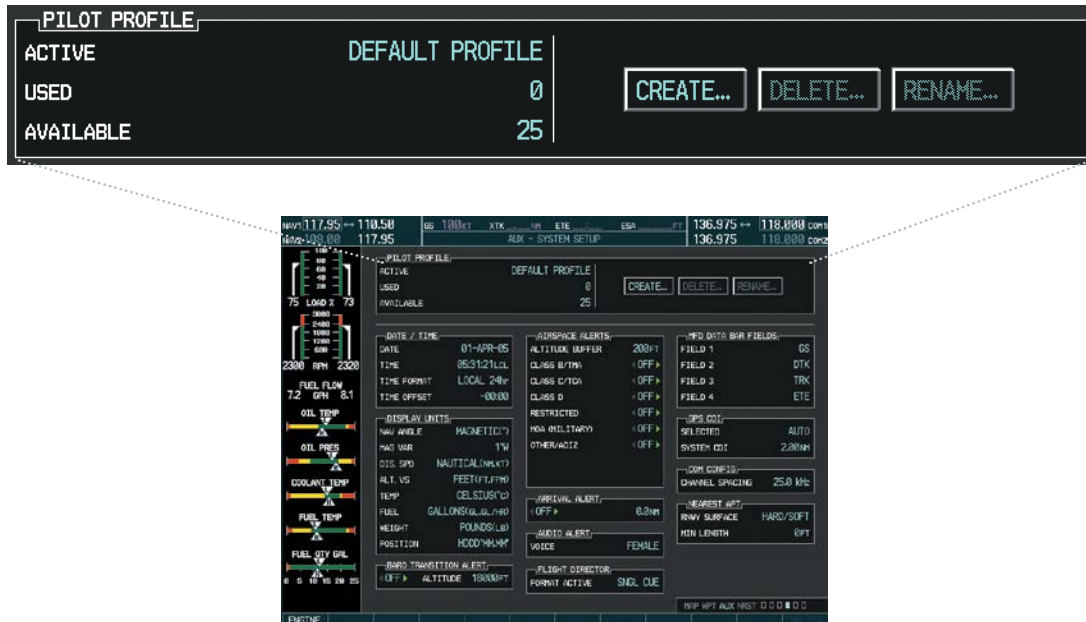
Figure 1-33 Display Unit Settings (AUX - System Setup Page)
