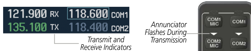
Figure 4-4 COM Radio Transmit and Receive Indications
