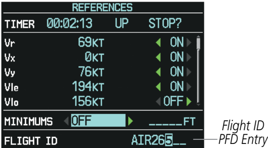
Figure 4-45 Timer/References Window, Entering Flight ID
