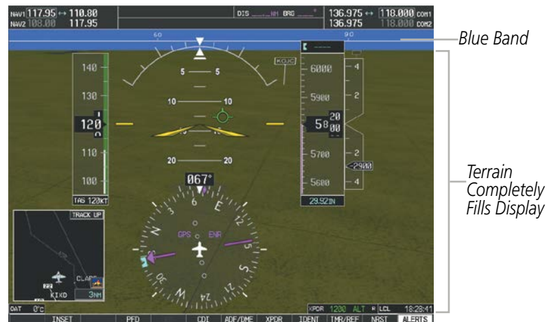
Figure 8-82 Blue Sky Bar with Full Display Terrain
