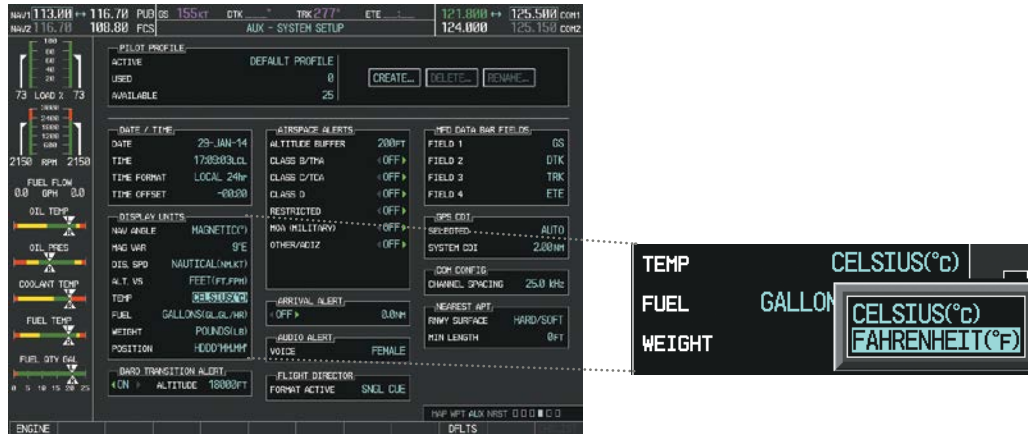
Figure 2-27 AUX-System Setup Page, Temperature Selection
