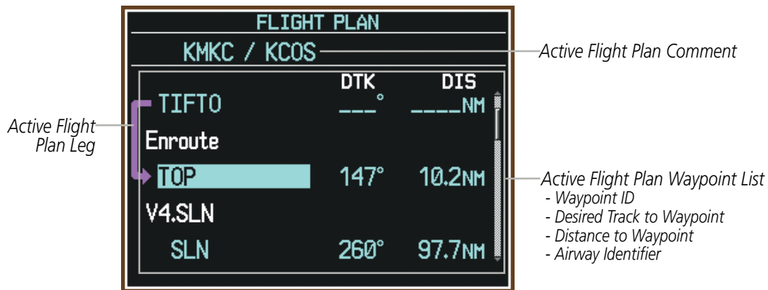
Figure 5-55 Active Flight Plan Window on PFD
