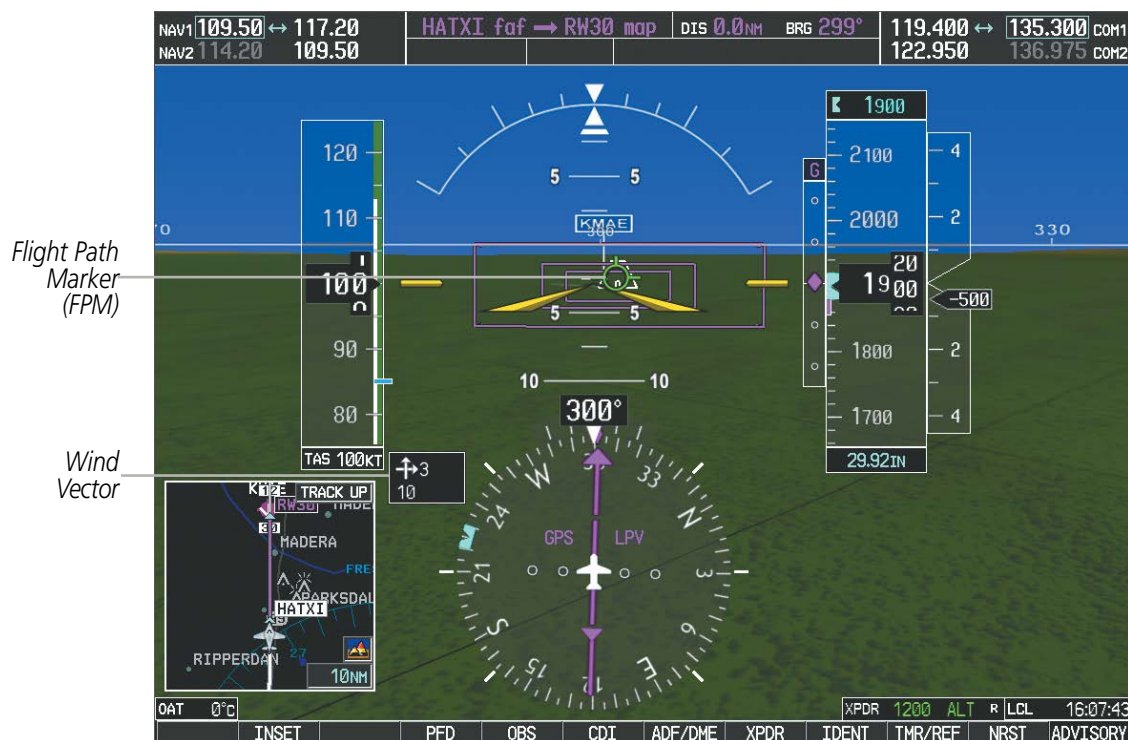
Figure 8-7 Flight Path Marker and Pathways
