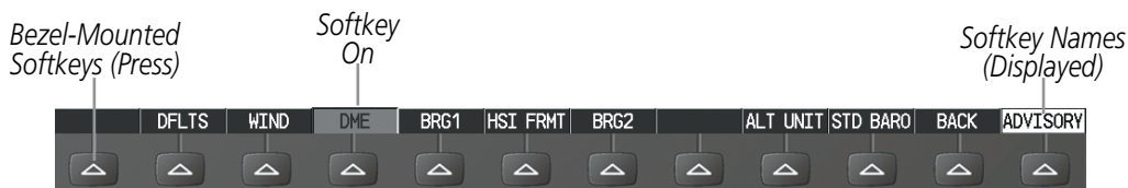
Figure 1-15 Softkeys (Second-Level PFD Configuration)
