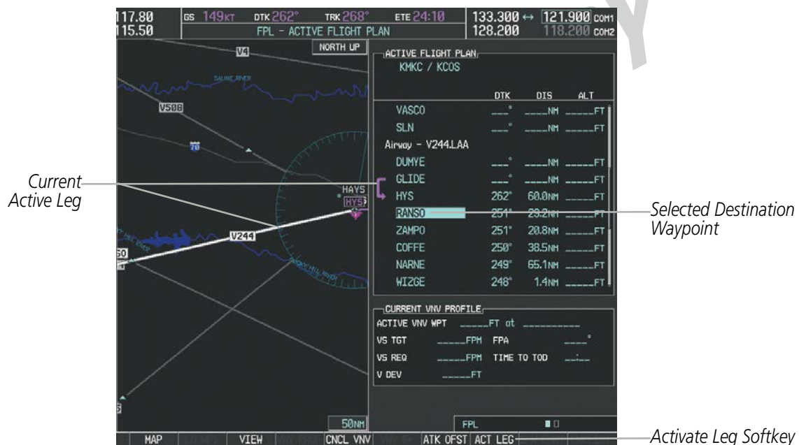
Figure 5-80 Active Flight Plan Page - Selecting the Leg Destination Waypoint
