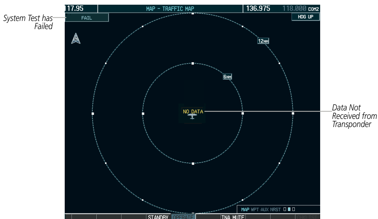
Figure 6-86 TIS Power-up Test Failure
