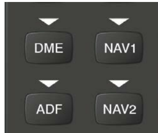
Figure 4-18 Selecting a NAV Radio Receiver
