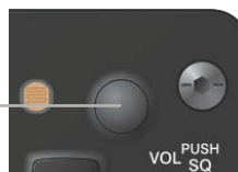
Figure 4-15 Overriding Automatic Squelch
