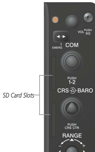
Figure 1-3 Display Bezel SD Card Slots
