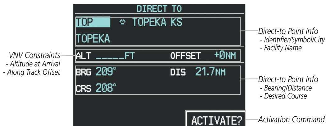
Figure 5-50 Direct-to Window - PFD
