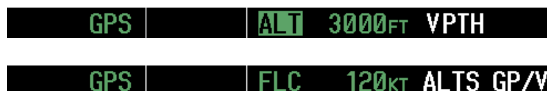
Figure 7-10 Vertical Path Tracking Armed Annunciations
