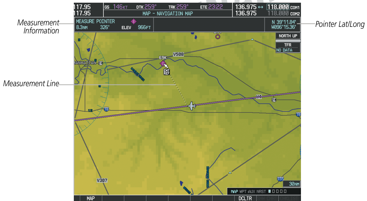
Figure 5-13 Navigation Map - Measuring Bearing and Distance
