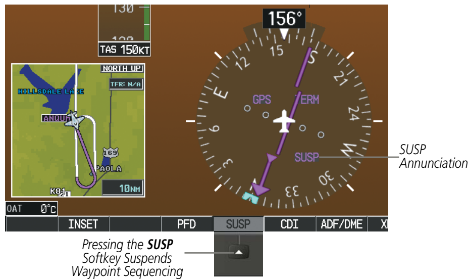
Figure 2-25 Suspending Automatic Waypoint Sequencing
