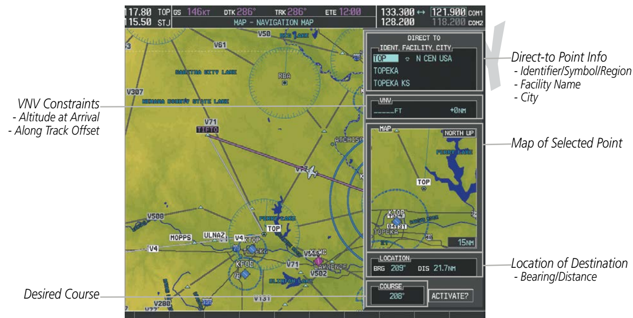
Figure 5-49 Direct-to Window - MFD
