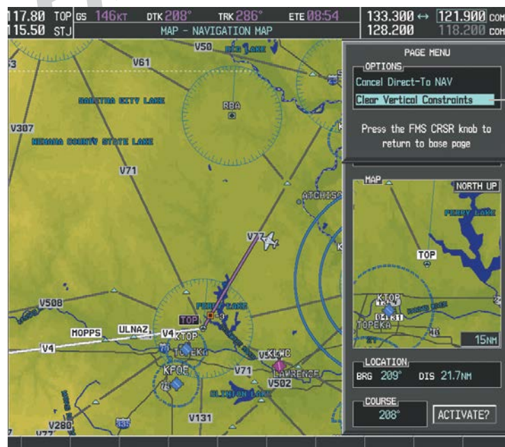
Figure 5-53 Direct-to Window - Clearing Vertical Constraints
