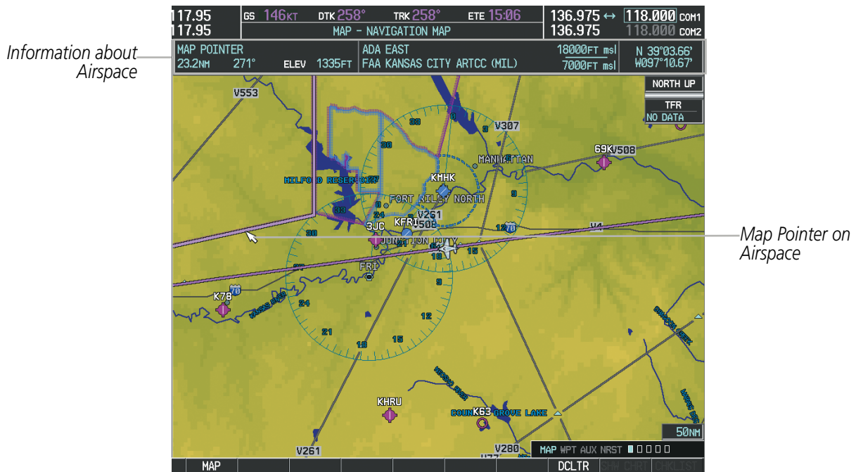
Figure 5-10 Navigation Map - Map Pointer on Airspace
