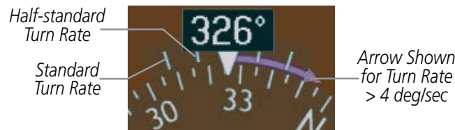
Figure 2-15 Turn Rate Indicator and Trend Vector
