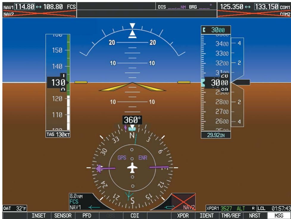
Figure 4-66 PFD1 Display after PFD2 Failure
