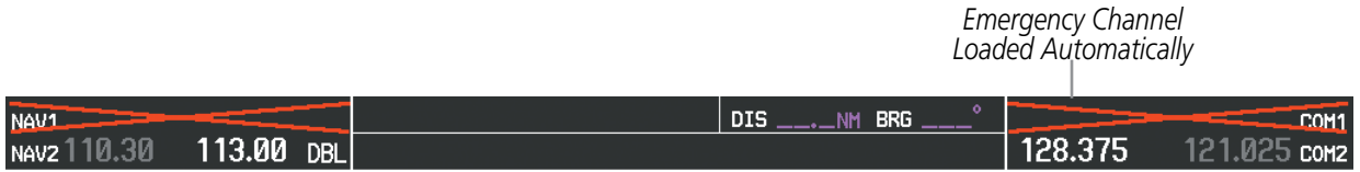
Figure 4-65 Frequency Section of PFD2 Display after PFD1 Failure
