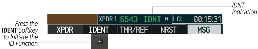
Figure 4-55 IDENT Softkey and Indication
