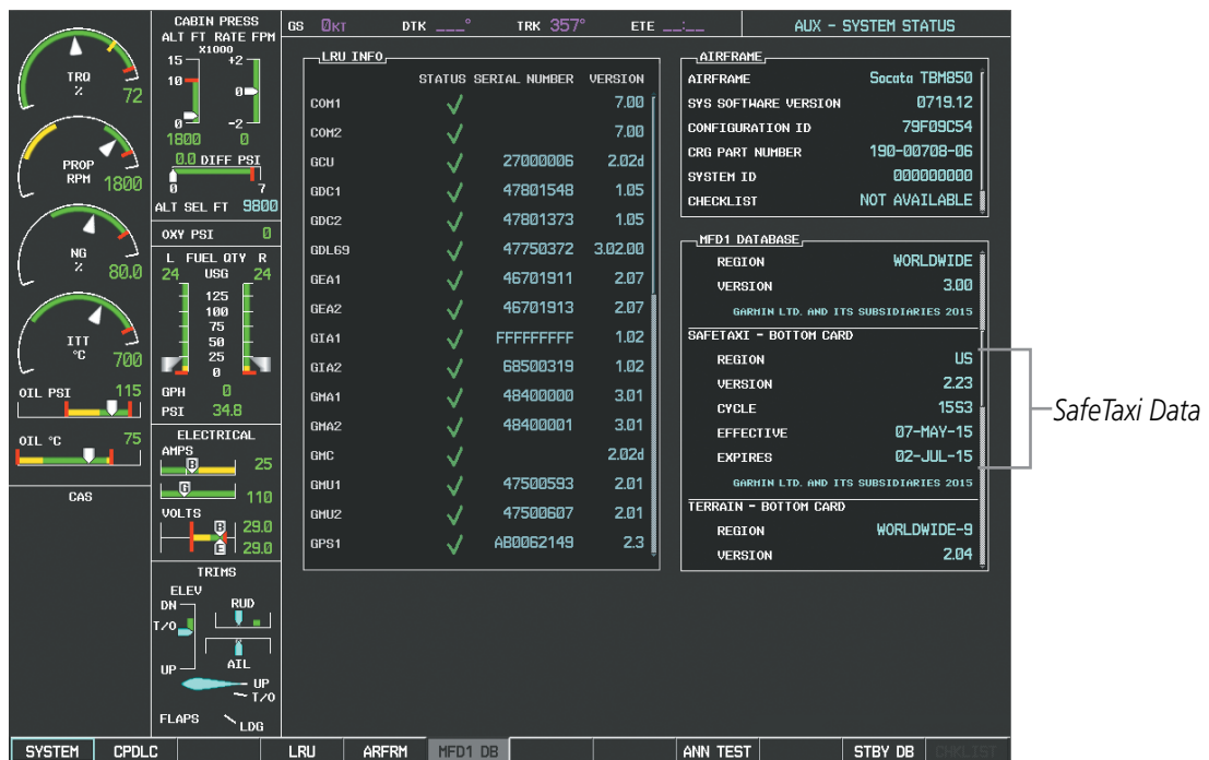
Figure 8-18 AUX – System Status Page, SafeTaxi Current Information
