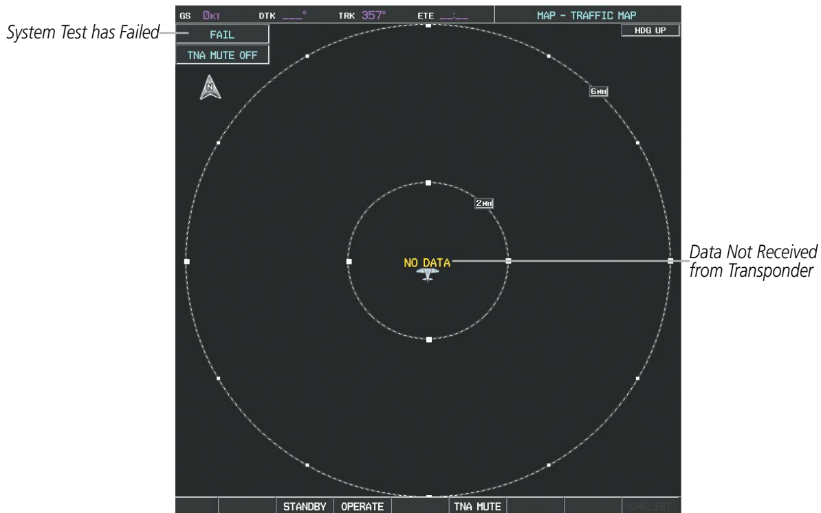
Figure 6-171 TIS Power-up Test Failure
