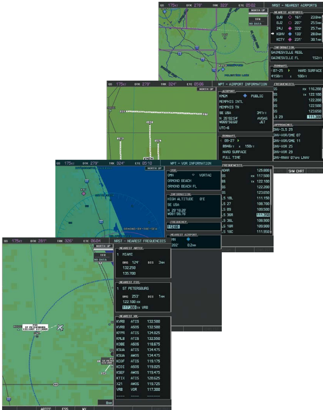
Figure 4-37 NRST – Nearest Frequencies, WPT – VOR Information, WPT – Airport Information, and NRST – Nearest Airports Pages
