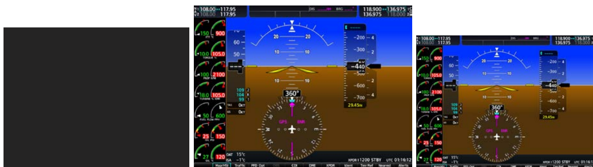
Figure 2-39, Manual Reversion with pilot PFD failure
