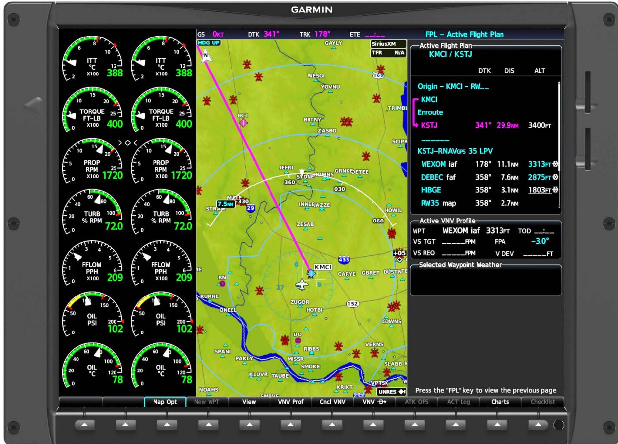
Figure 20, Display of Temperature-Compensated Altitudes
