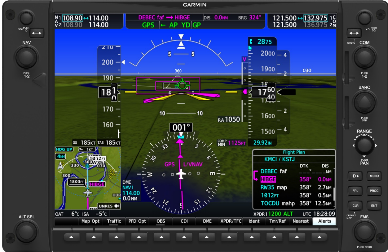
Figure 23, Vertical Deviation Display With Barometric Approach Vertical Guidance
