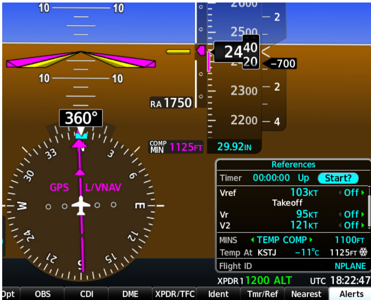
Figure 21, Temperature Compensation of Minimum Altitude
