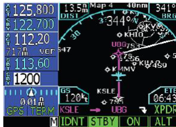
Figure 3-5 GNS 480 Transponder Control
