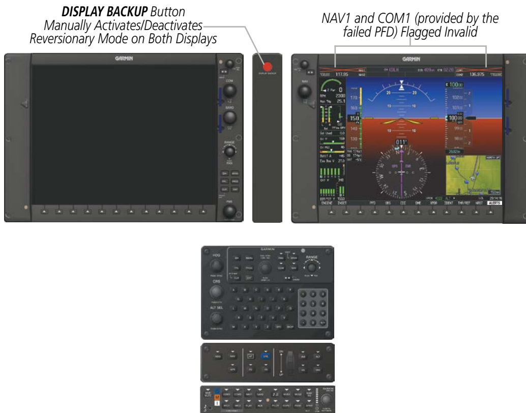
Figure 1-17 Reversionary Mode (Failed PFD)
