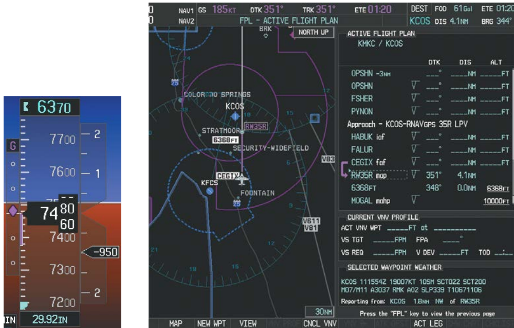
Figure 5-157 Descending to the Missed Approach Point
