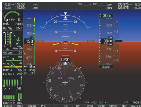
Figure 2-28 Outside Air Temperature
