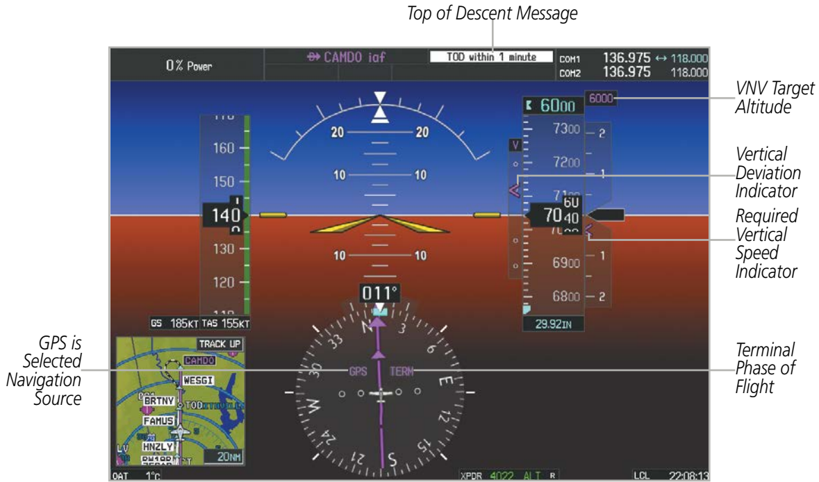
Figure 2-32 Vertical Navigation Indications (PFD)
