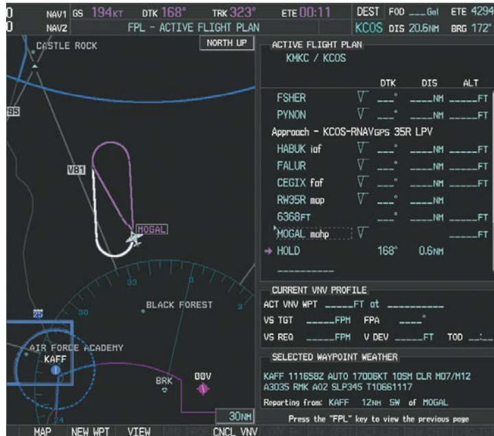
Figure 5-159 Establishing the Holding Pattern
