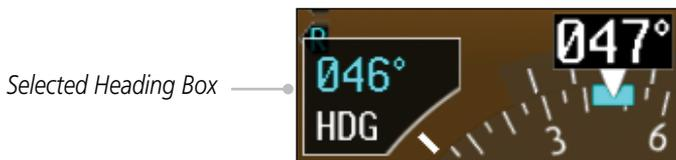
Figure 5-28 Adjusting the Heading Bug
