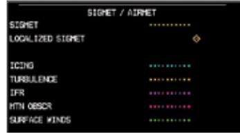
**Figure 4-103 GFDS Weather - AIRMETS/SIGMETs Detail and Legend**
