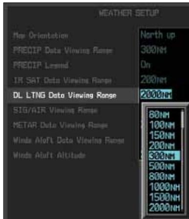
Figure 4-101 GFDS Lightning Viewing Range Selection
