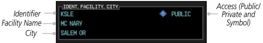
**Figure 3-119 Flight Plan Ident/Facility/City Detail**
