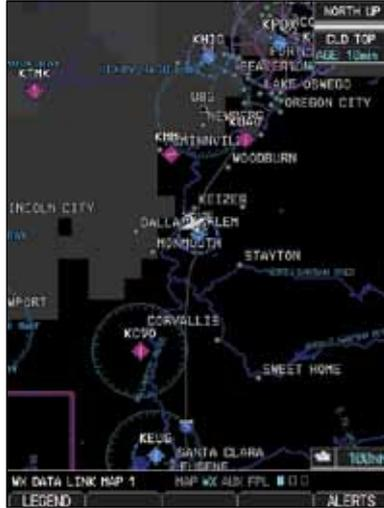
Figure 4-31 XM Weather - Cloud Tops
