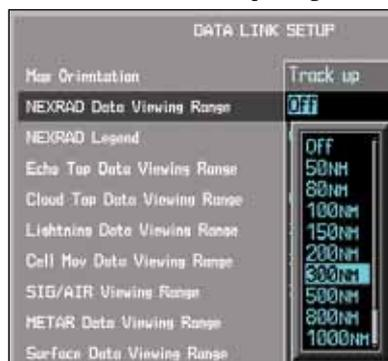
Figure 4-27 NEXRAD Viewing Range Selection
