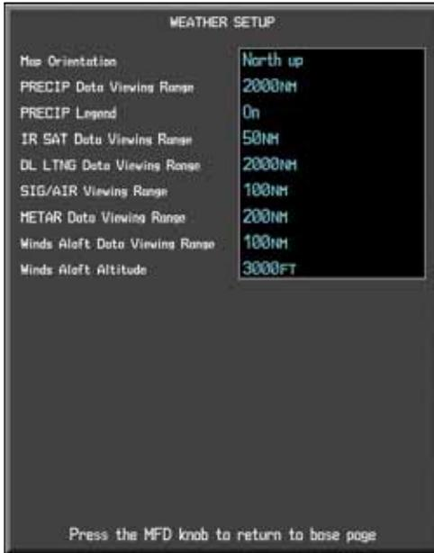
**Figure 4-85 Weather Data Link Setup Menu Options**
