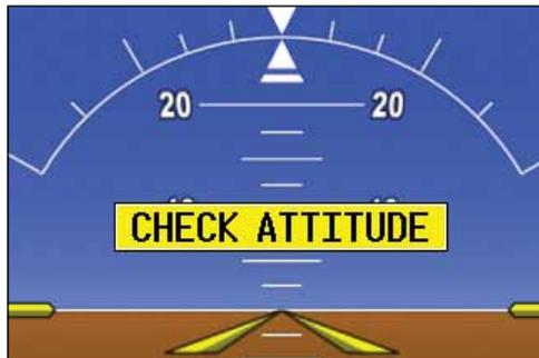
Figure 5-27 Check Attitude - Autopilot Automatically Disconnected
