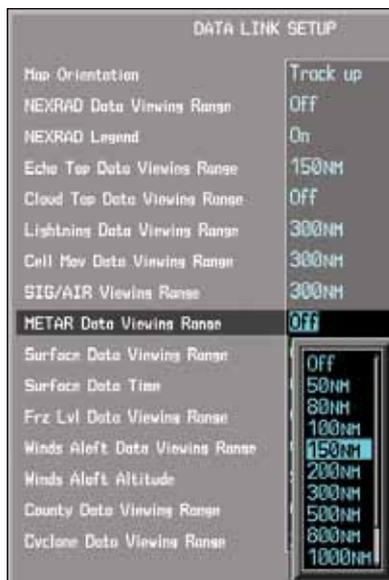
**Figure 4-40 METAR Viewing Range Selection**
