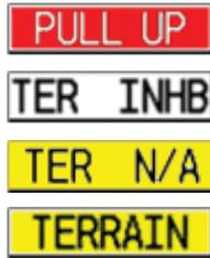
Figure 4-10 TAWS Annunciations from a GNS/GTN TAWS
