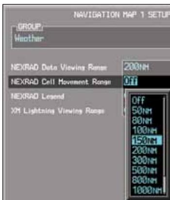
**Figure 3-46 NEXRAD Cell Movement Selection**
