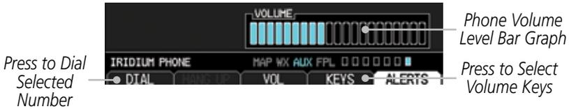
**Figure 3-105 Select Soft Keys for Phone Volume Adjustment**
