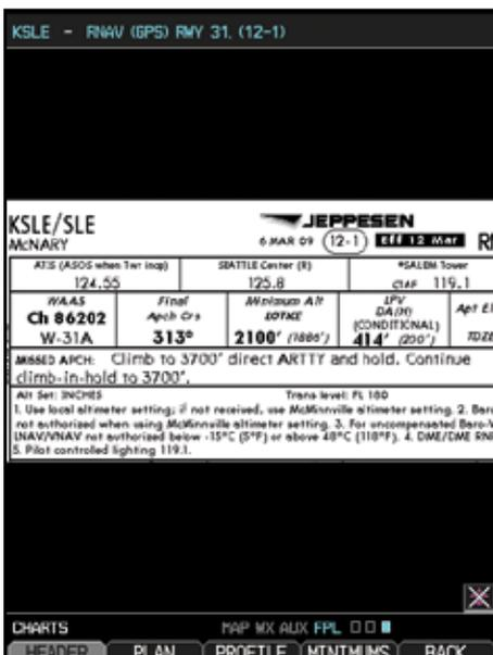
Figure 5-14 Detail of the Selected Chart (Header Shown)
