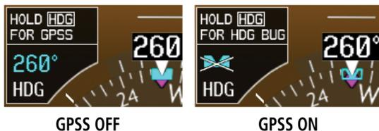
Figure 5-31 GPSS mode control with the HDG key
