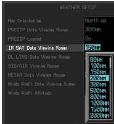
**Figure 4-99 GFDS IR SAT Viewing Range Selection**
