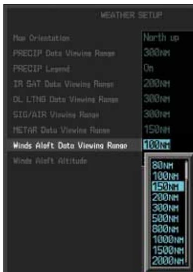
**Figure 4-109 Winds Aloft Data Viewing Range Selection**
