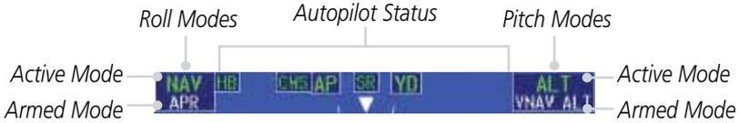
**Figure 5-35 Autopilot Annunciations on Top of PFD**
