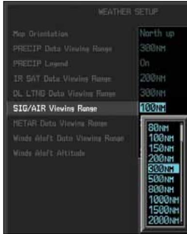
Figure 4-104 GFDS SIG/AIR Viewing Range Selection
