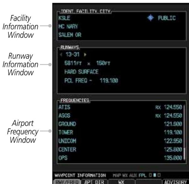
Figure 3-118 Flight Plan Waypoint Info Detail
