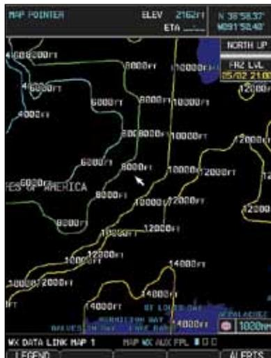
Figure 4-48 XM Weather - Freezing Levels
