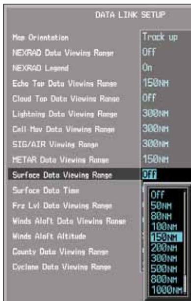
**Figure 4-46 Surface data Viewing Range Selection**
