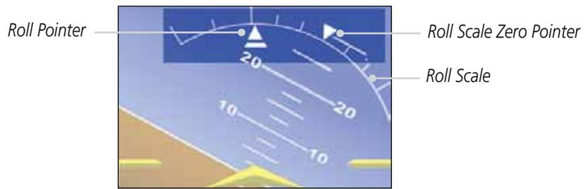
**Figure 2-14 Attitude Indicator with a Ground Pointer configuration in a left turn**
