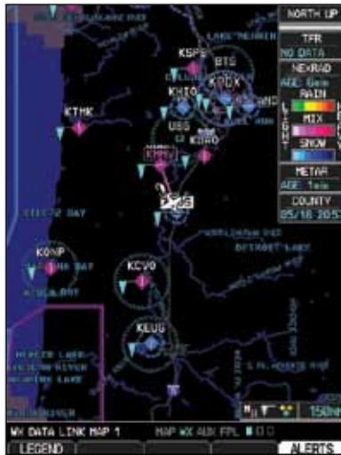
Figure 4-39 XM Weather - Graphic METARs
