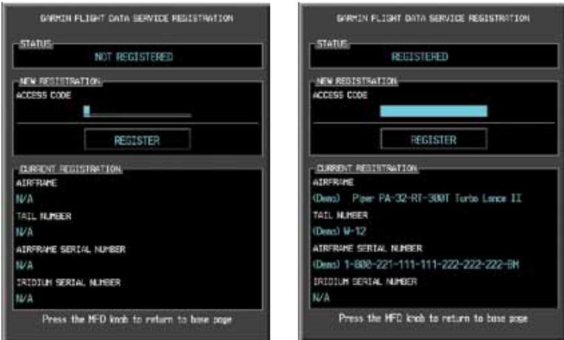
**Figure 4-83 GFDS Registration Page (Default and Completed)**
