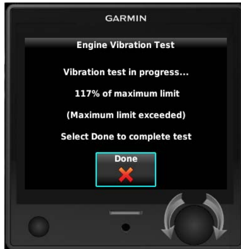
Figure 5-1 Engine Vibration Test Failure Indication
