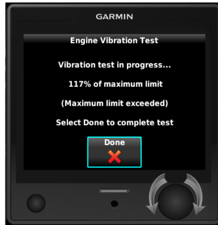
Figure 6-3 Engine Vibration Test Failure Indication
