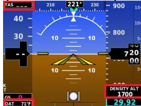
Figure 6-4 ADI display of OAT and TAS (typical values shown)
