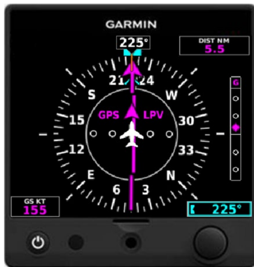
Figure 1-3 G5 Electronic Flight Instrument (DG/HSI)
