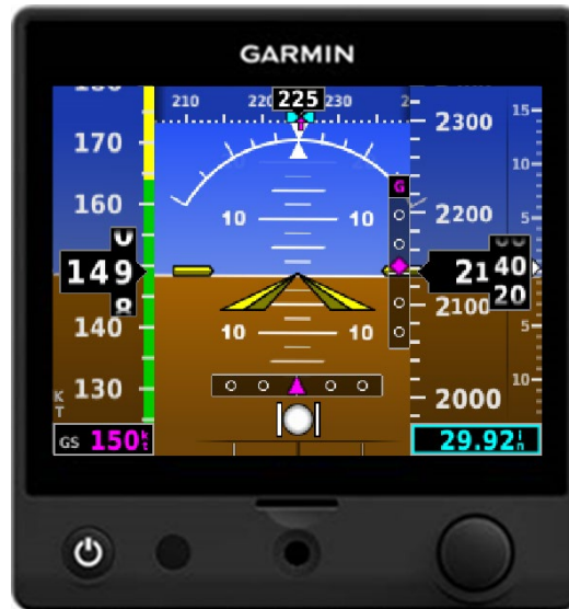
Figure 1-1 G5 Electronic Flight Instrument (Attitude)
