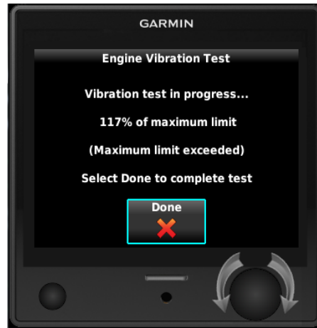
Figure 6-3 Engine Vibration Test Failure Indication
