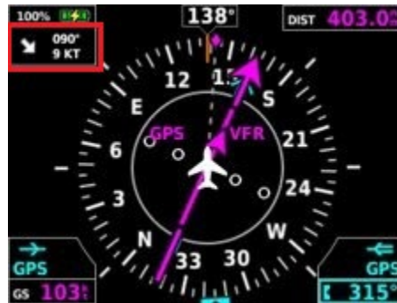
Figure 6-5 HSI Display of Crosswind (Typical Values Shown)
