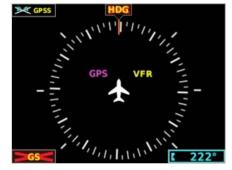
Figure 1-3 G5 HSI Page Failure Annunciations
