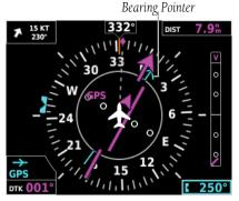
Figure 2-16 GPS Source Bearing Pointer
