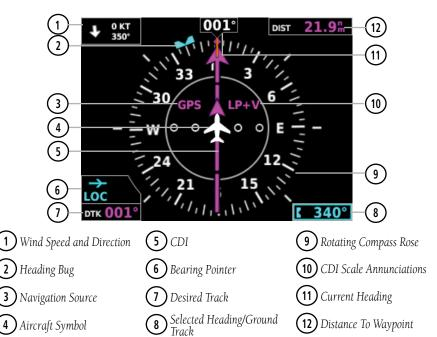
Figure 2-15 Horizontal Situation Indicator (HSI)
