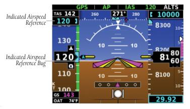
Figure 3-13 Indicated Airspeed Reference on PFD Page
