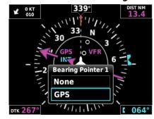
Figure 2-20 Bearing Pointer Source Options
