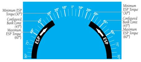
Figure 3-28 ESP Roll Operating Range When Engaged (Force Increases as Roll Increases & Decreases as Roll Decreases)
