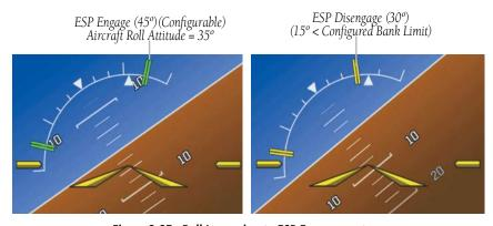
Figure 3-27 Roll Increasing to ESP Engagement
