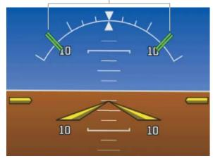
Figure 3-26 ESP Roll Engagement Indication (ESP Enabled but NOT Engaged)
