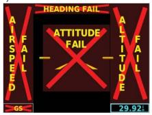
Figure 1-2 G5 PFD Page Failure Annunciations
