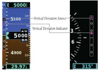
Figure 2-25 Vertical Deviation Indicator (Glidepath GPS Source) - PFD
