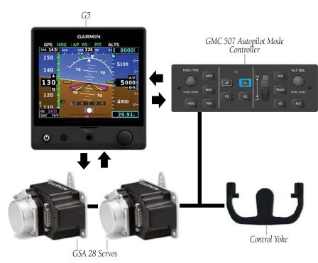
Figure 3-1 Core GFC 500 System
