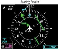
Figure 2-17 VOR Source Bearing Pointer
