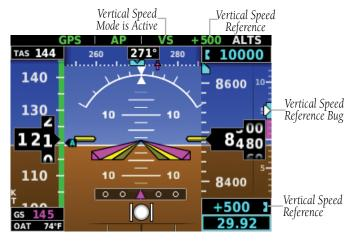
Figure 3-11 Vertical Speed Reference on PFD Page
