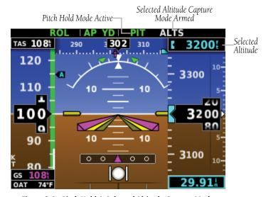
Figure 3-8 Pitch Hold & Selected Altitude Capture Modes
