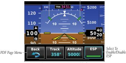
Figure 3-25 AFCS (ESP Enabled)
