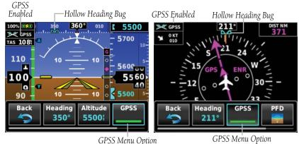
Figure 4-3 GPSS Enabled - PFD
