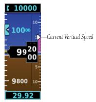
Figure 2-14 Vertical Speed Indicator
