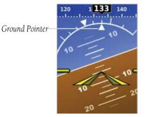
Figure 2-7 Ground Pointer Configuration
