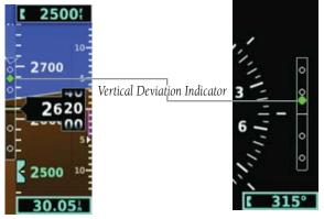
Figure 2-23 Vertical Deviation Indicator (Glideslope ILS Source) - PFD
