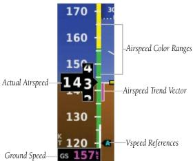
Figure 2-2 Airspeed Indicator
