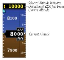
Figure 2-10 Altitude Alerting Visual Annunciation
