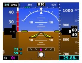
When GPSS is selected on the G5, GPSS turn commands are converted into a heading error signal to the autopilot. When the autopilot is operated in HDG mode, the autopilot will fly the turn commands from the GPS
