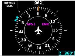
1. Use an alternate source of outside air temperature to calculate true airspeed, density altitude, and winds.
