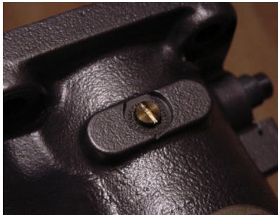
Figure 21-20 Carb Temp Sensor Mounting Location
