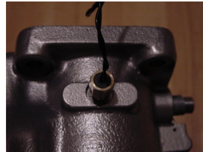
Figure 21-22 Carb Temp Sensor Installed
