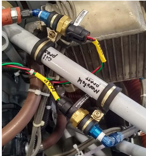
Figure 21-12 Pressure Transducer Mounting
