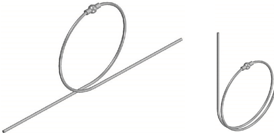
Figure 30-22 360° and 540° Cable Wrap Examples
