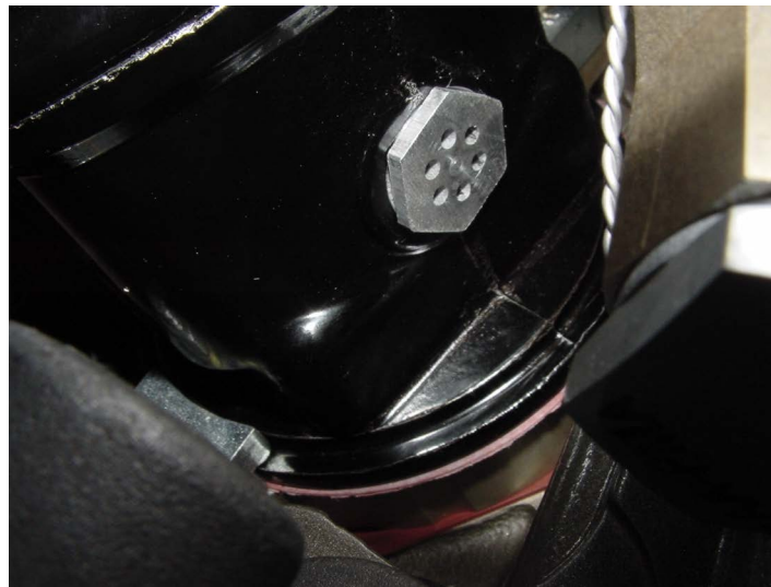
Figure 21-15 Magneto Bleed Port
