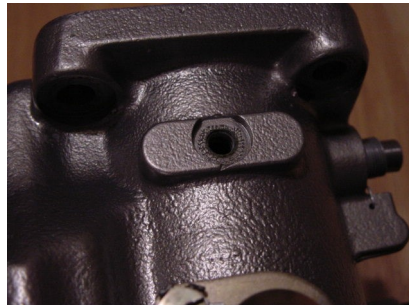
Figure 21-21 Carb Temp Sensor Mounting Location w/Screw Removed
