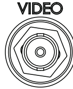
Figure 23-10 View of Video Input BNC Connector from Back of Unit
