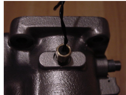
Figure 21-22 Carb Temp Sensor Installed
