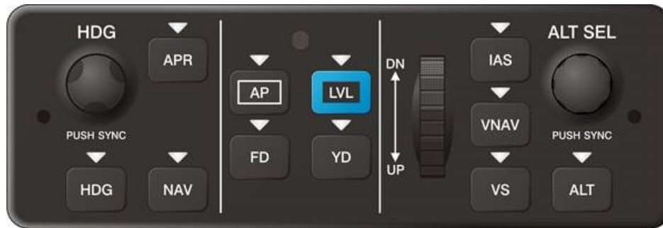
Figure 11-1 GMC 307 Unit View (-00 version shown, -20 version has no YD button)
