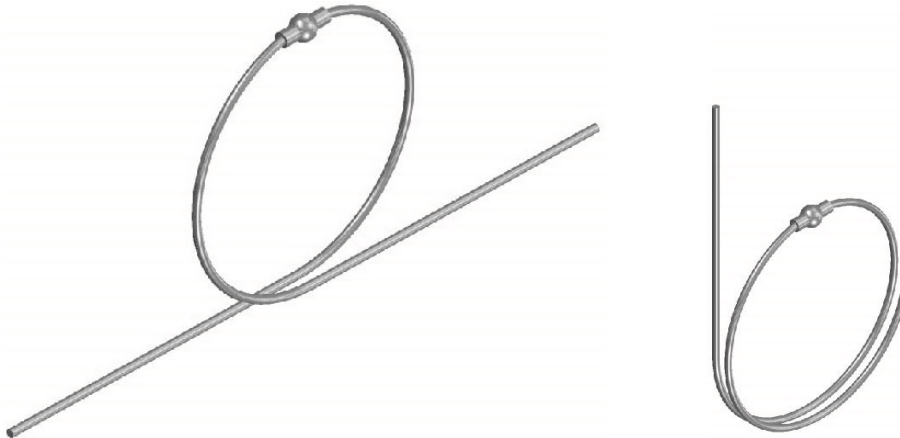
Figure 30-22 360° and 540° Cable Wrap Examples
