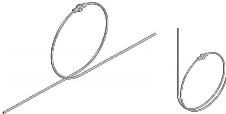
Figure H-4 360° and 540° Cable Wrap Examples
