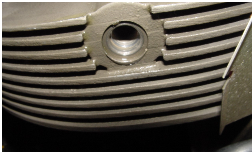
Figure 21-4 CHT Probe Well
