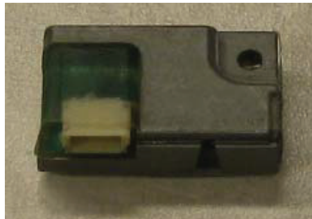
Figure 2-2 Original Green Configuration Module P/N 011-00979-20
