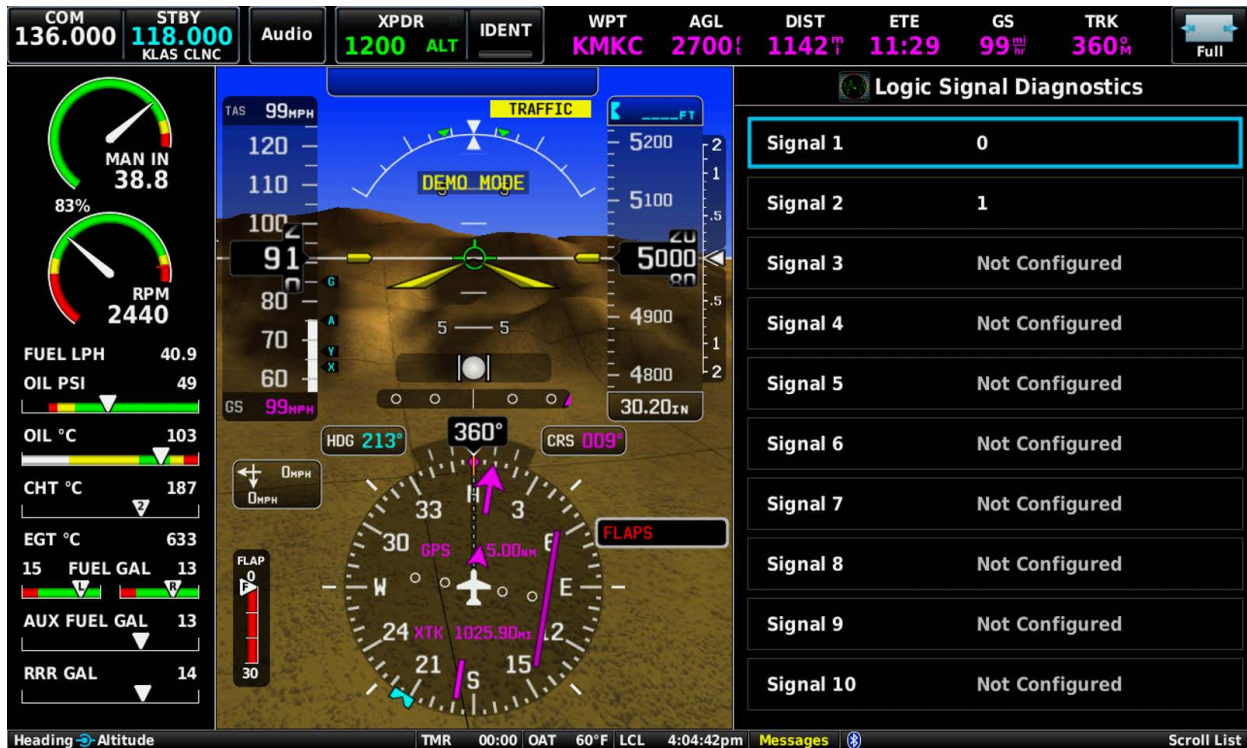
Figure 30-73 Logic Signal Diagnostics Page
