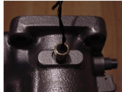
**Figure 21-22 Carb Temp Sensor Installed**
