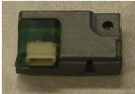
**Figure 2-2 Original Green Configuration Module P/N 011-00979-20**
