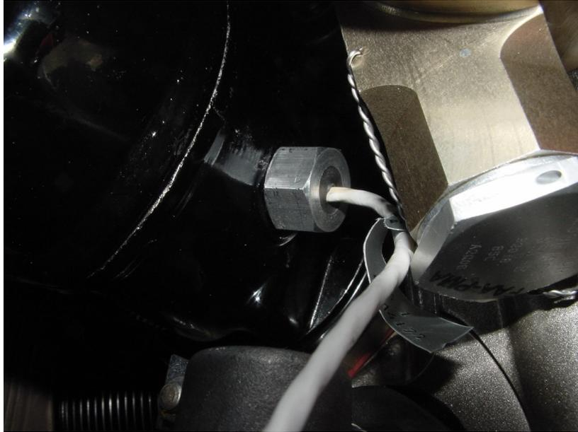
**Figure 21-17 Magneto Tach Sensor Installed**
