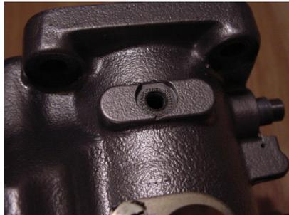
**Figure 21-21 Carb Temp Sensor Mounting Location w/Screw Removed**
