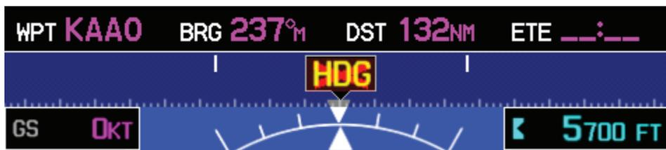
**Figure 31-4 Heading Failure Indication (Full-Screen PFD)**
