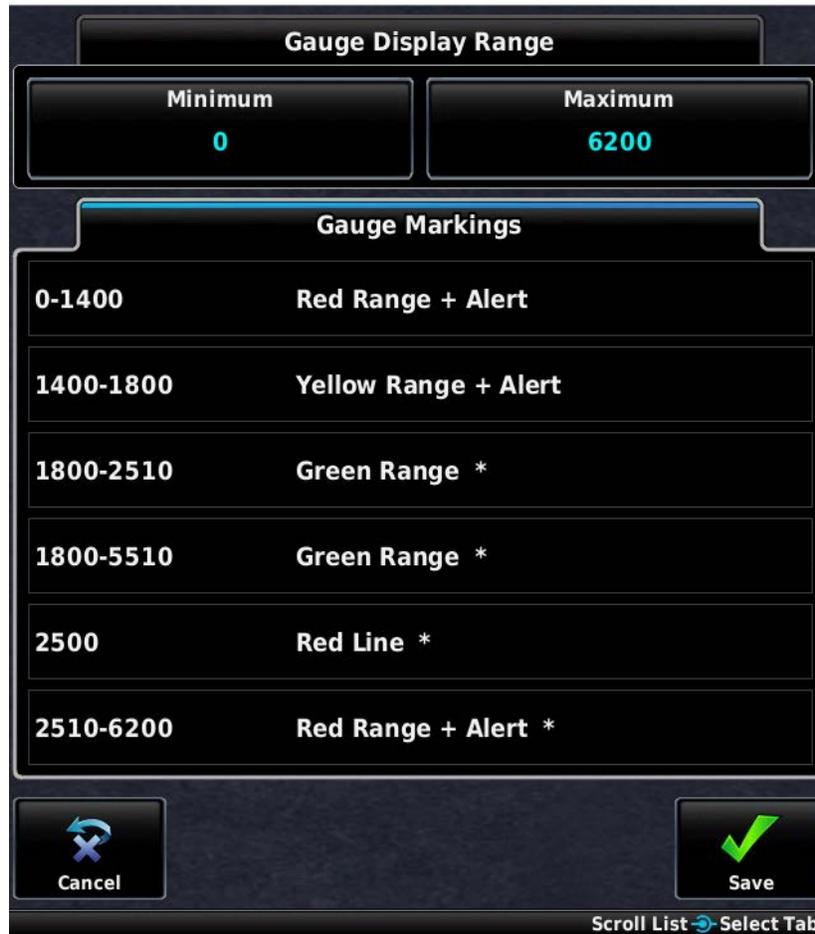
Figure 30-68 Gauge Markings List Showing Use Of Logic Signals
