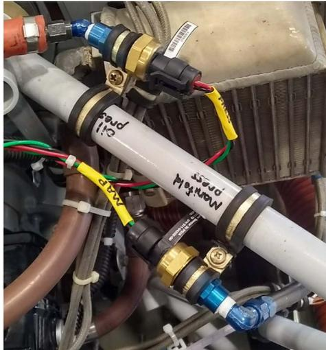
**Figure 21-12 Pressure Transducer Mounting**
