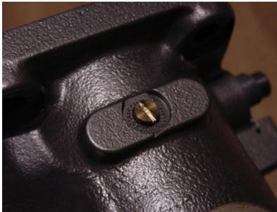
**Figure 21-20 Carb Temp Sensor Mounting Location**
