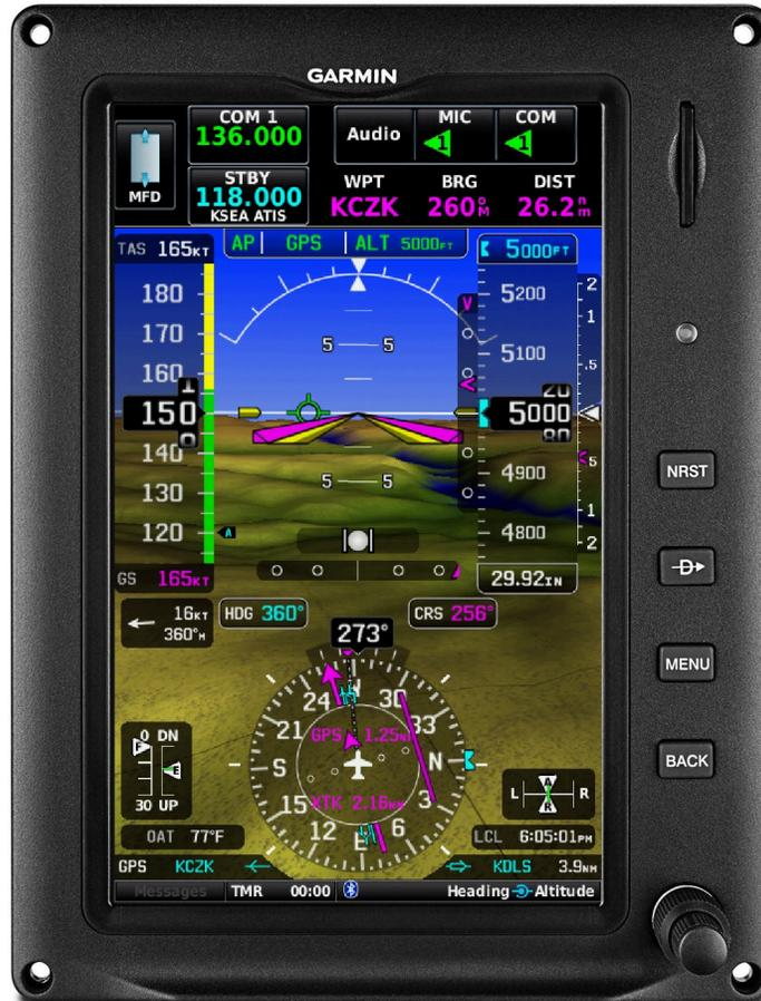
Figure 6-3 GDU 470 Unit View
