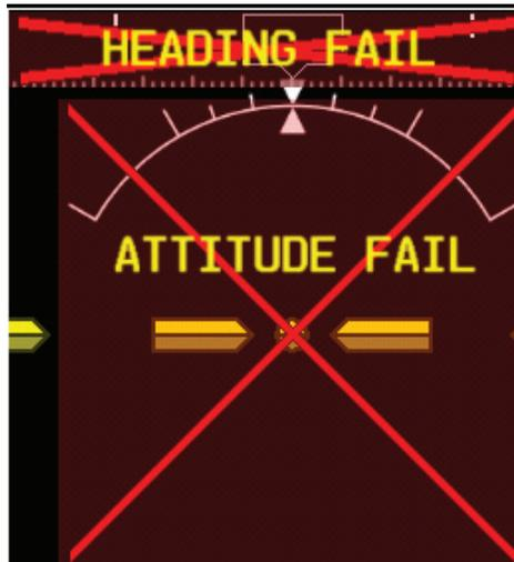
**Figure 31-5 Attitude and Heading Failure Indications (Reversionary or Split-Screen PFD)**
