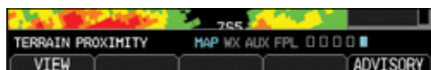
Figure 4-1 Terrain Page with VIEW Soft Key to reach 360° and 120° Arc Soft Keys
