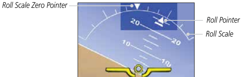
Figure 2-12 Attitude Indicator with a Sky Pointer Configuration in a Left Turn
