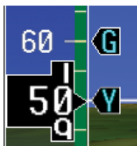
V Speed References on Airspeed Tape
