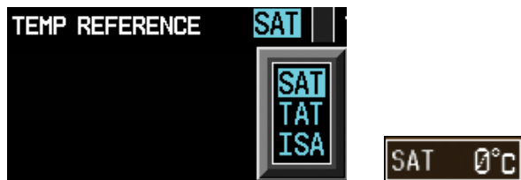
Figure 3-44 Outside Air Temperature Selection
