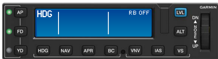
GMC 605 Annunciating Smart Rudder Bias Off (RB OFF)
