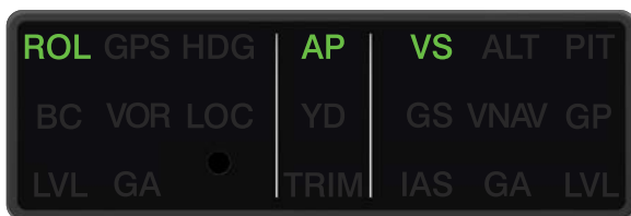
GI 285 Annunciating Vertical Speed Mode
