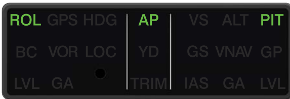
GI 285 Annunciating Roll Hold Mode
