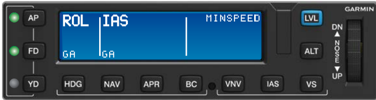
GMC 605 Underspeed Indication (Altitude Critical Mode)
