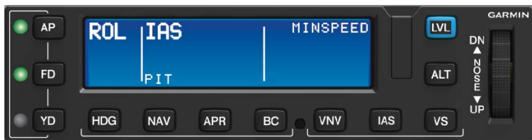
GMC 605 Underspeed Indication (Non-Altitude Critical Mode)
