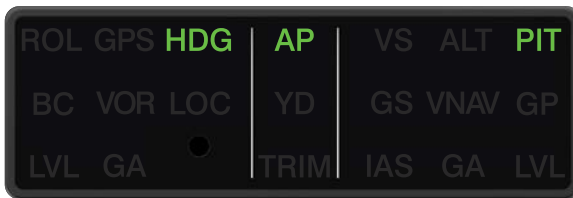
GI 285 Annunciating Heading Mode
