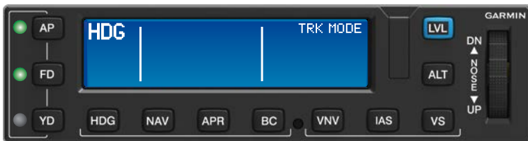
GMC 605 Annunciating Reversionary GPS Track Mode
