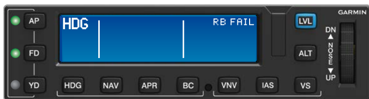
GMC 605 Annunciating Smart Rudder Bias Fail (RB FAIL)
