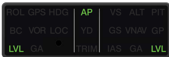
GI 285 Annunciating Level Mode
