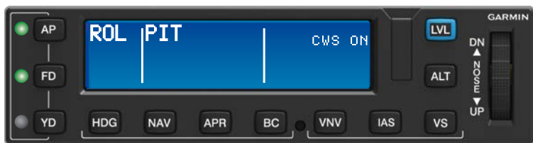
GMC 605 Annunciating Control Wheel Steering
