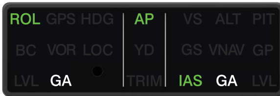
GI 285 Underspeed Indication (Altitude Critical Mode)
