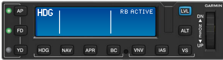
GMC 605 Annunciating Smart Rudder Bias Active
