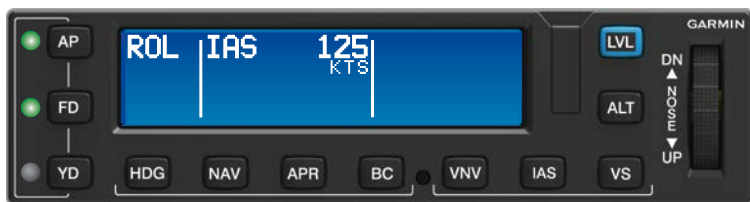
GMC 605 Annunciating Indicated Airspeed Mode
