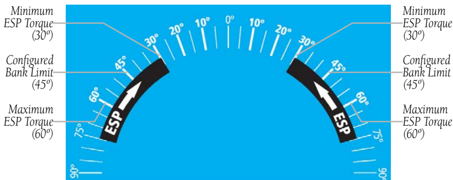
ESP Roll Operating Range When Engaged (Force Increases as Roll Increases & Decreases as Roll Decreases)
