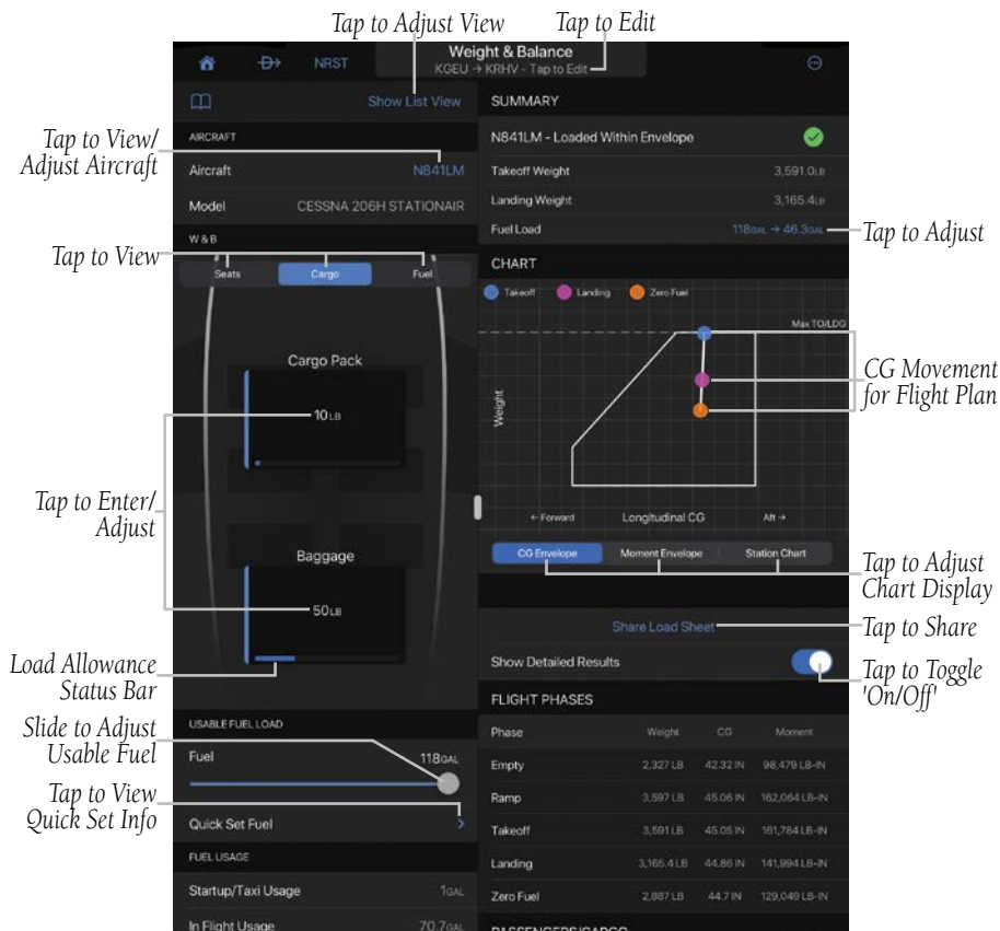
Weight and Balance - Airplane - Graphical View - Cargo - Data Entered
