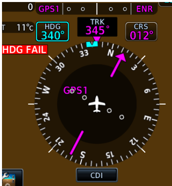
HSI with Magnetometer Failure
