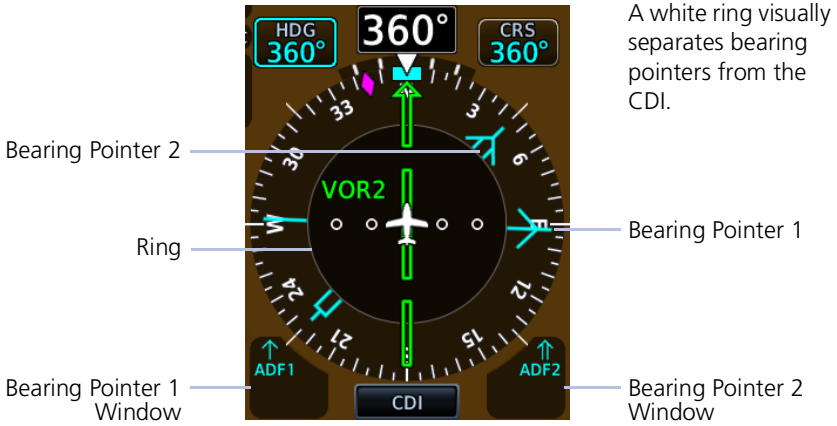
GDU 1060/700P, Dual Bearing Pointers
