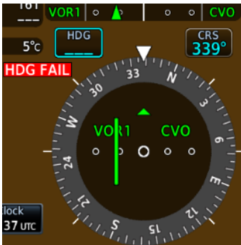
HSI with GPS and Magnetometer Failures
