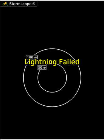
Stormscope Alert Annunciation
