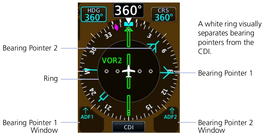
Dual Bearing Pointers, GDU 700P/1060
