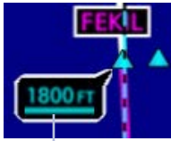
Altitude Constraint Label
