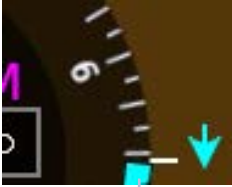
Heading Bug Off Scale
