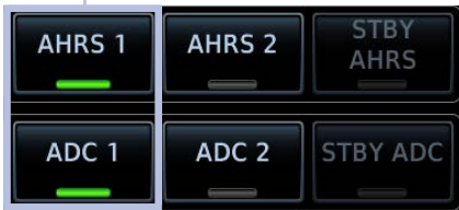
Pilot Selected Sensors (Active)
