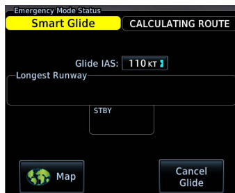
Smart Glide Active, Calculating Route
