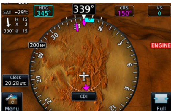
Engine Annunciator on PFD
