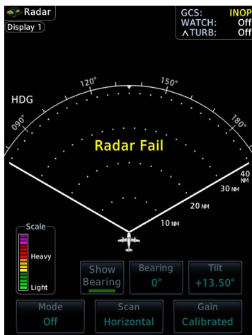
Radar Alert Annunciation
