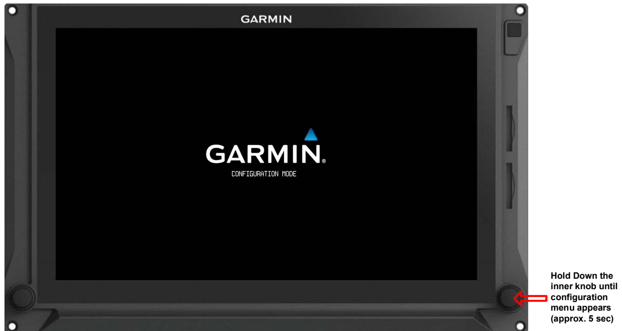
Figure 2-1 Entering the Configuration Mode on the GDU
