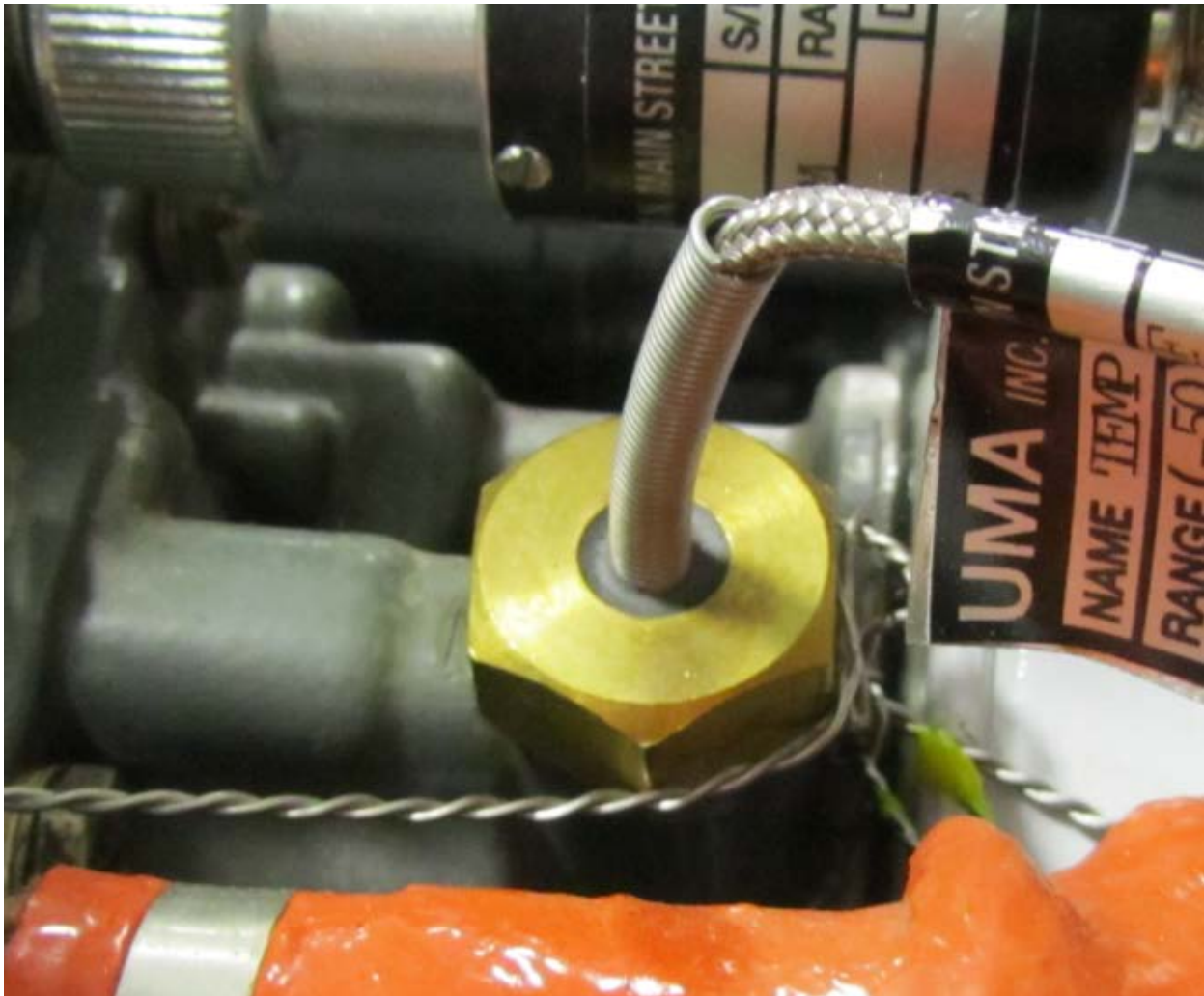
Figure 5-25 Oil Temperature Sensor Installation Example
