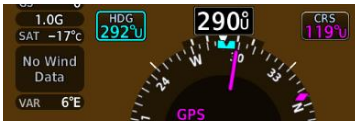
Figure 4-4: User Navigation Angle with magnetic variation (VAR) set to 6°E
