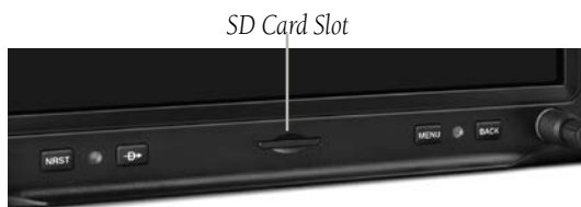
SD Card Slot - GDU 46X (10.6 inch)
