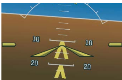
ESP Engaged (Nose-Low)
