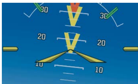
ESP Engaged (Nose-High)
