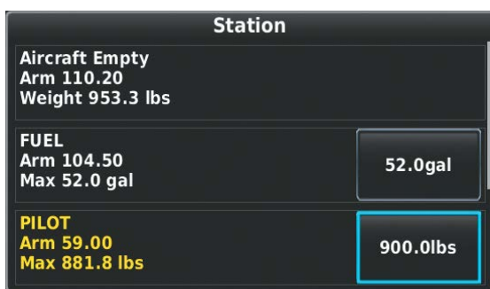
Loading Limit Exceeded
