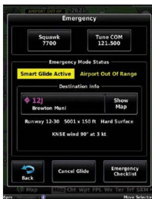
Airport Out of Range (Emergency Page)
