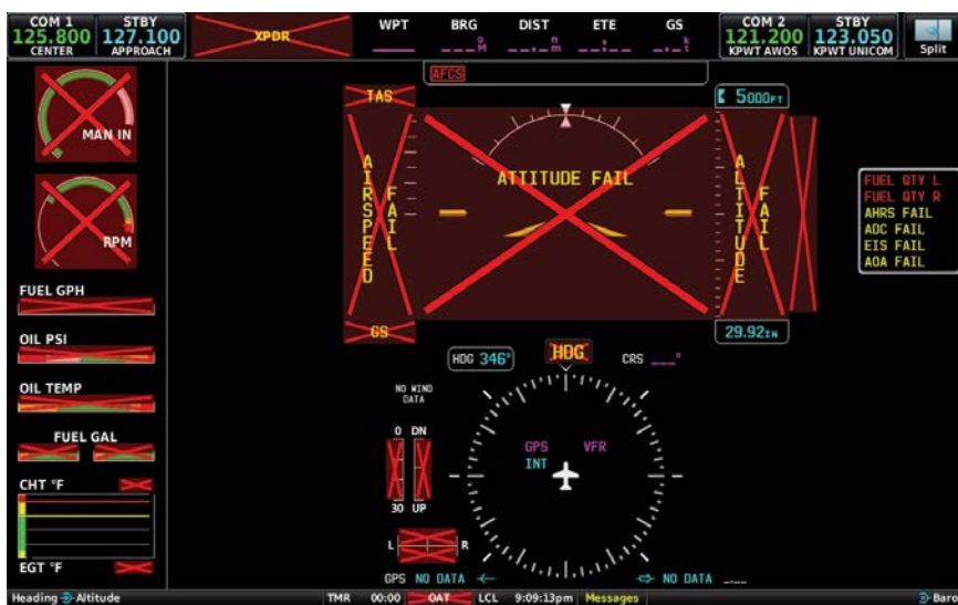
G3X Touch System Failure Annunciations
