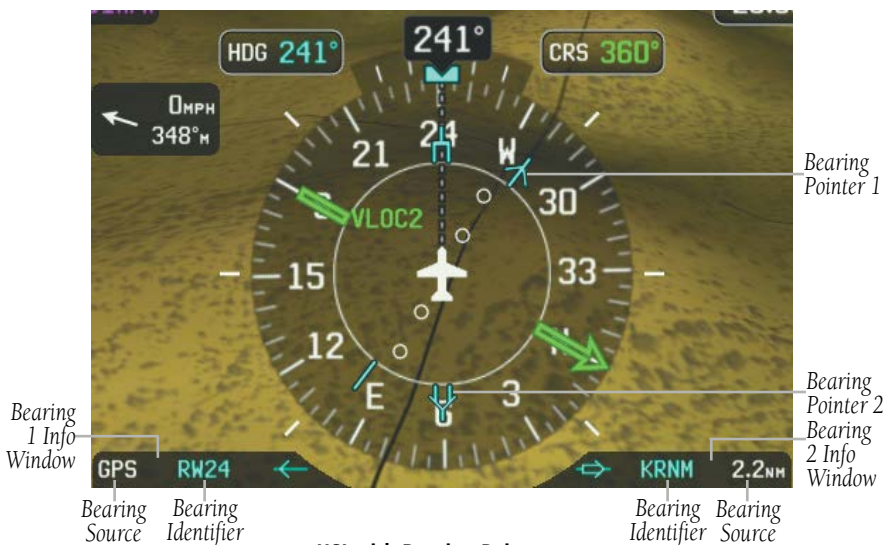
HSI with Bearing Pointers
