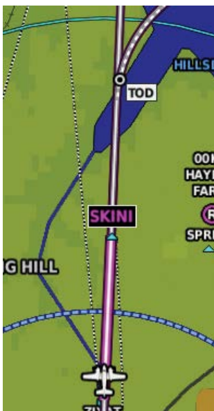
Top of Descent Indication (Available when Configured with a GTN Xi Only)
