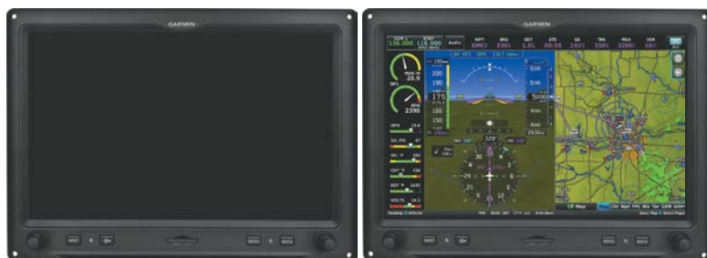
G3X Touch Full-Screen Reversionary Mode (Failed PFD)
