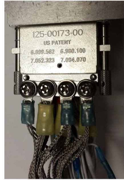
Figure 3-13 GMA 245R Audio Shield Termination (top and bottom)
