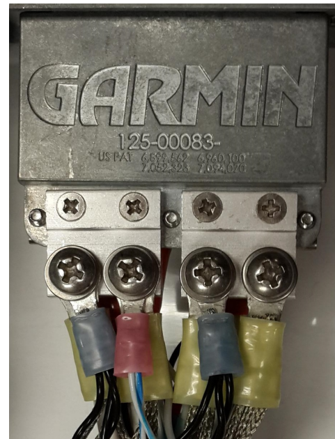
Figure 3-12 GMA 245 Audio Shield Termination (top and bottom)
